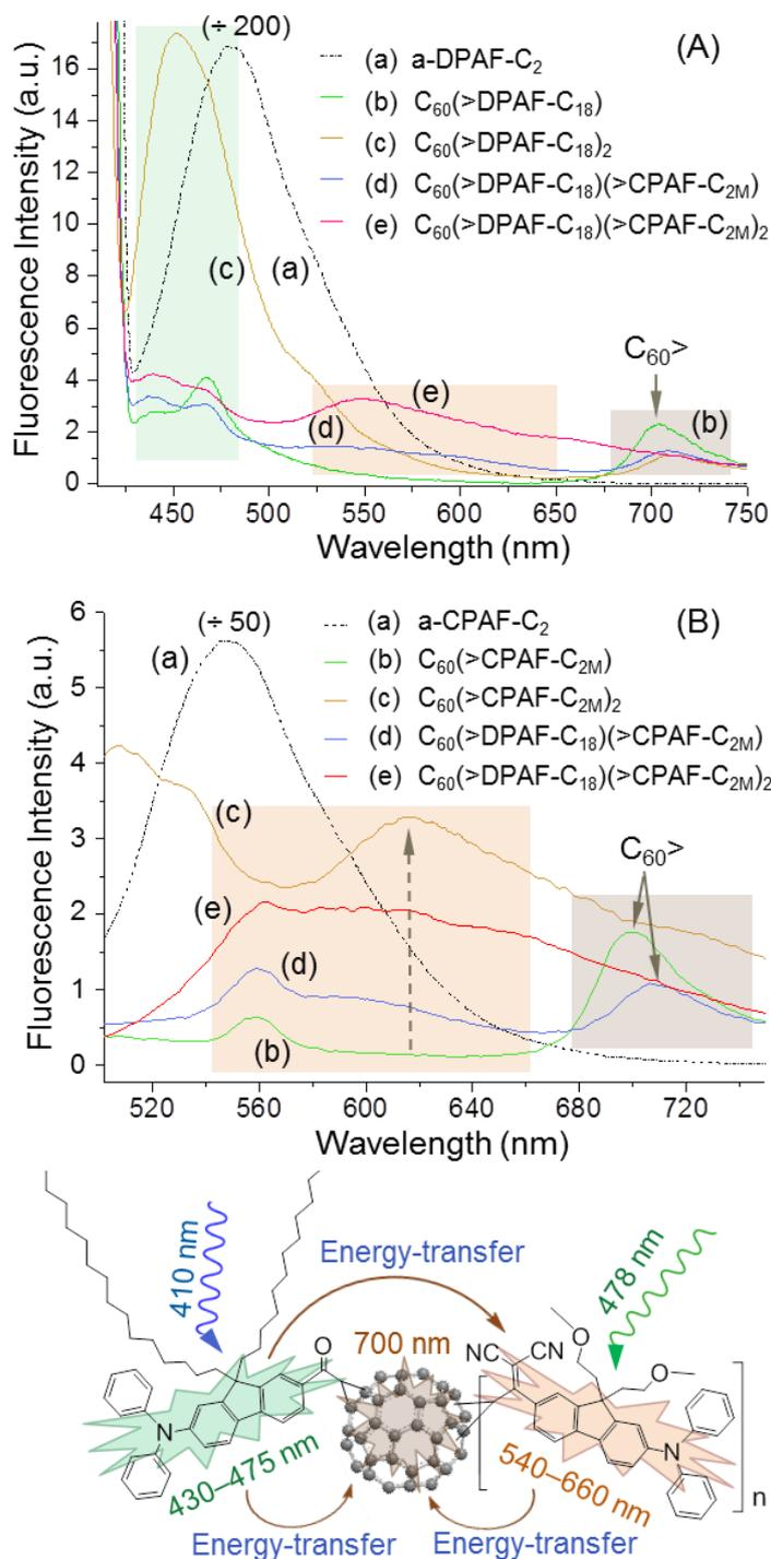
Interestingly, upon photoexcitation of the triad **3** specifically on the DPAF- $C_{18}$  antenna moiety at 410 nm, the resulting FL spectrum [Figure 7A(d)] displayed a weak broad FL band at 448 [from  $^1(DPAF)^*-C_{18}$ ] and broad bands at 525–650 nm along with the  $^1(C_{60}>)^*$  emission band centered at 708 nm. The latter broad bands fit in the similar range as those of  $C_{60}[>^1(CPAF)^*-C_{2M}]_2$ . As the number of
