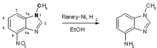
Heterocyclic amines [1] can be prepared from the corresponding nitro-group containing compounds by catalytic or chemical reduction [2].
