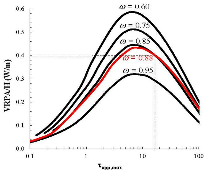
**Figure 6.** Effect of the maximum optical thickness on the VRPA per unit of length of a CPC solar reactor. Adapted from Colina-Marquez *et al.* [37].
