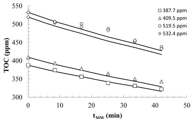
**Figure 9.** Validation of the TOC photocatalytic degradation with 0.4 g/L of catalyst load.
