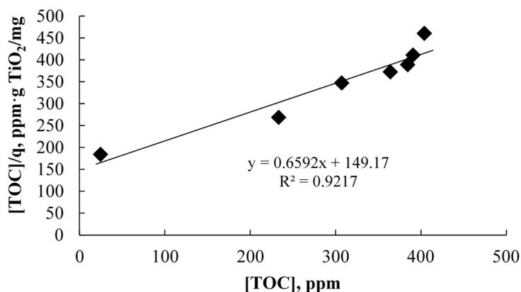
**Figure 4.** Linear regression of the Langmuir isotherm obtained from experiments at 30 °C, pH 6.9 and with 0.6 g/L of catalyst load.
