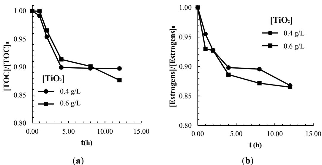
**Figure 3.** Adsorption of commercial estradiol at 0.4 and 0.6 g/L of catalyst loading with an initial concentration of 7 ppm of estrogens and 429 ppm of TOC: (a) TOC removal and (b) Estrogens removal.
