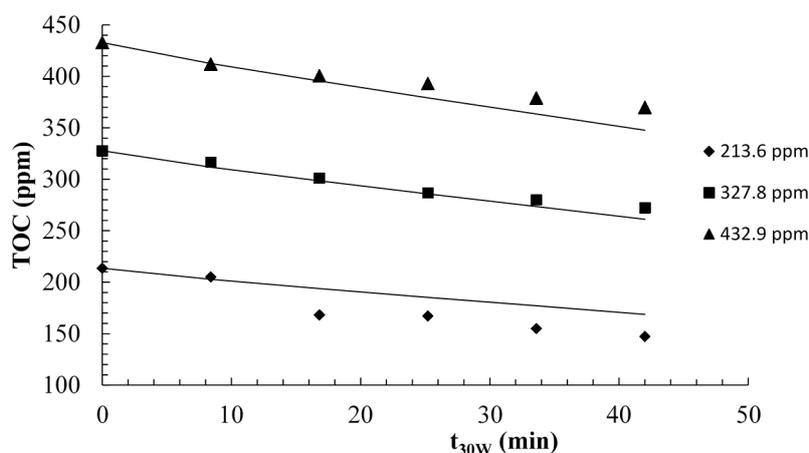
**Figure 8.** Modeling of the photocatalytic mineralization of commercial estradiol. The initial pH was 4.6 and the catalyst loading was 0.6 g/L.
