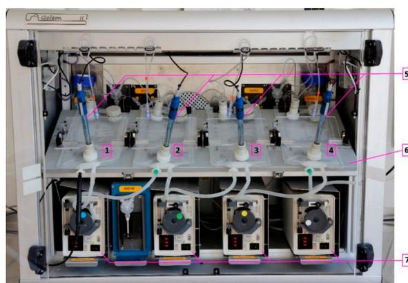
**Figure 1.** Golem v2 apparatus photographed from the front view: (1) stomach, (2) duodenum, (3) jejunum, (4) ileum, (5) pH probes, (6) heating platform, and (7) peristaltic pumps.
