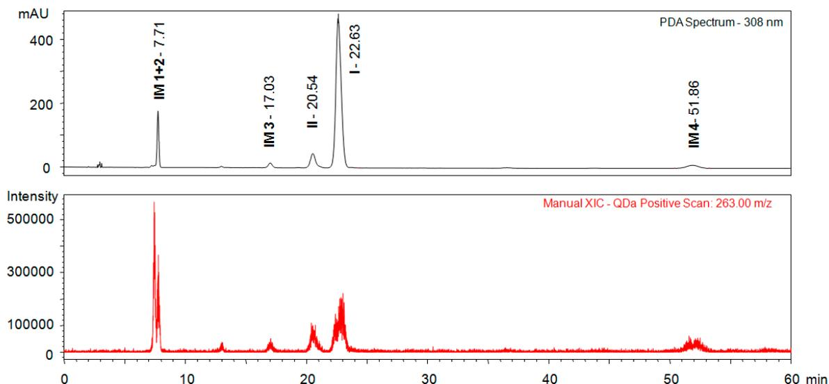
**Figure S-4.** Identification of an impurity located at 7.71 min. Conditions: ChiralArt Amylose-C (250×4.6 mm, i.d., 5  $\mu$ m) column, mobile phase scCO<sub>2</sub>/IPA (70/30), flow rate of 1 mL/min, sample concentration 1.0 mg/mL, injection volume 10  $\mu$ L, temperature 30 °C, backpressure 2000 psi, ESI+.
