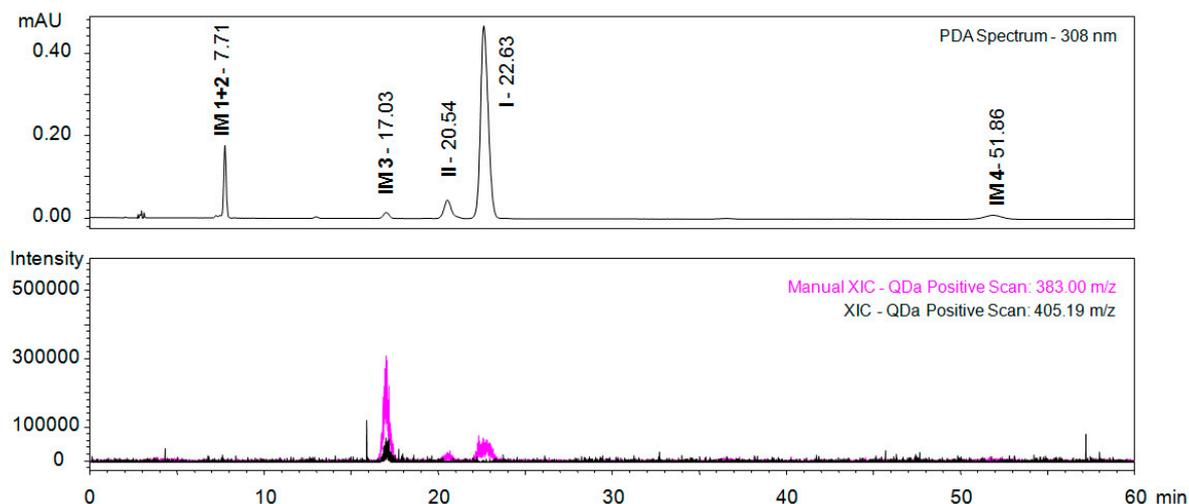
**Figure S-8.** Identification of the third impurity located at 17.03 min,  $[M+H]^+$  383.0 Da and 405.2  $[M+Na]^+$ . Conditions: ChiralArt Amylose-C (250×4.6 mm, i.d., 5  $\mu$ m) column, mobile phase  $scCO_2$ /IPA (70/30), flow rate of 1 mL/min, sample concentration 1.0 mg/mL, injection volume 10  $\mu$ L, temperature 30 °C, backpressure 2000 psi, ESI+.
