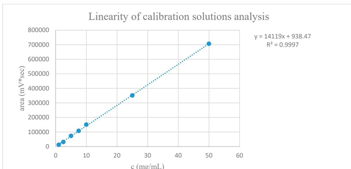
Figure S-3. Linear regression for the first measurements of calibration solutions.
