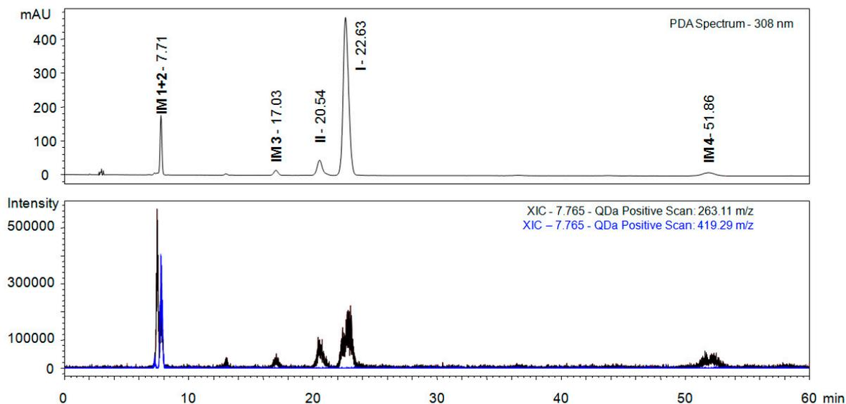
**Figure S-5.** Identification of the second impurity located at 7.71 min. Conditions: ChiralArt Amylose-C (250×4.6 mm, i.d., 5 μm) column, mobile phase scCO<sub>2</sub>/IPA (70/30), flow rate of 1 mL/min, sample concentration 1.0 mg/mL, injection volume 10 μL, temperature 30 °C, backpressure 2000 psi, ESI+.
