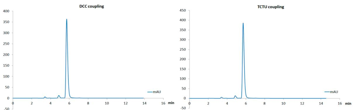
**Figure S-2.** Enantiomeric purity control of building blocks, prepared using two different coupling reagents, performed on Chiralpak AD-3 using ECOM HPLC; mobile phase heptane/propan-2-ol (9/1, v/v), flow rate 1 mL/min, temperature 25 °C, sample concentration 0.2 mg/mL, injection volume 20 μL.
