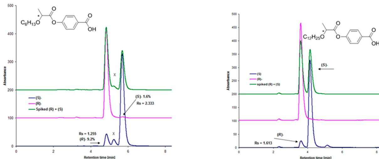
**Figure S-1.** Comparison of enantioseparation of **2a** and **2c** (left) with that of **2b** and **2d** (right) on Chiralpak® AD-3 (150×4.6 mm i.d., 4.6 μm) using ECOM HPLC in a heptane/IPA (9/1, v/v) mixture at the flow rate of 1 mL/min and temperature 25 °C. Sample concentration was 0.2 mg/mL, injection volume 20 μL and detection wavelength was set to 235 nm. Only synthetic methods (B) and (C) are shown.
