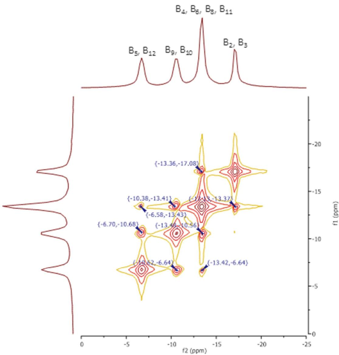
**Figure S6.** The two-dimensional  $^{11}\text{B}$ - $^1\text{H}$ - $^{11}\text{B}$ - $^1\text{H}$  COSY NMR spectra with the assigned boron vertices.
