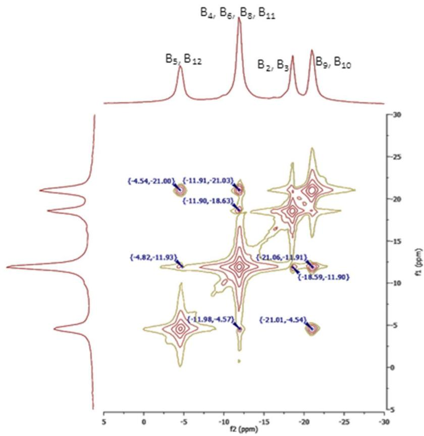
**Figure S13.** The two-dimensional  $^{11}\text{B}$   $\{{}^1\text{H}\}$ - $^{11}\text{B}$   $\{{}^1\text{H}\}$  COSY NMR spectra with the assigned boron vertices.
