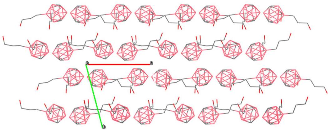
**Figure S30.** Crystal packing of the 9,10-(HOCH<sub>2</sub>CH<sub>2</sub>CH<sub>2</sub>)<sub>2</sub>-1,7-*clos*o-C<sub>2</sub>B<sub>10</sub>H<sub>10</sub> structure.
