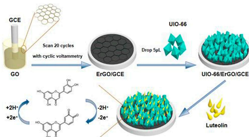
**Scheme 1.** The fabrication of UiO-66/ErGO/GCE and electrochemical detection of luteolin (LU).
