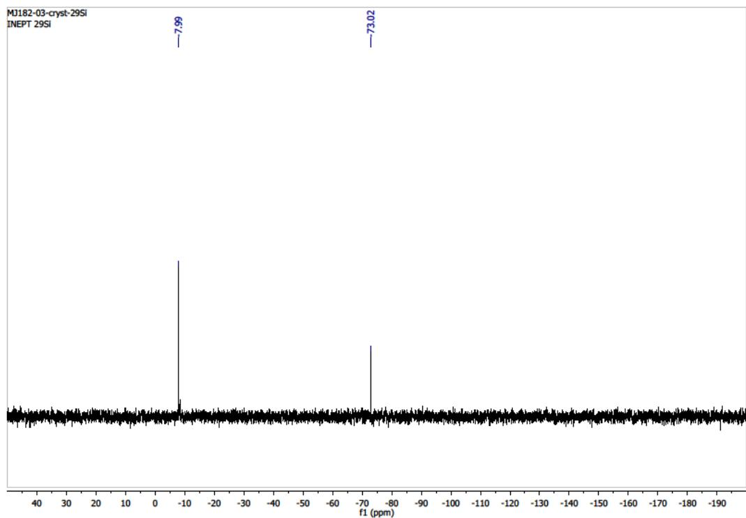
**Figure 9.**  $^{29}\text{Si}\{\text{H}\}$  INEPT NMR spectrum of **4** in  $\text{C}_6\text{D}_6$
