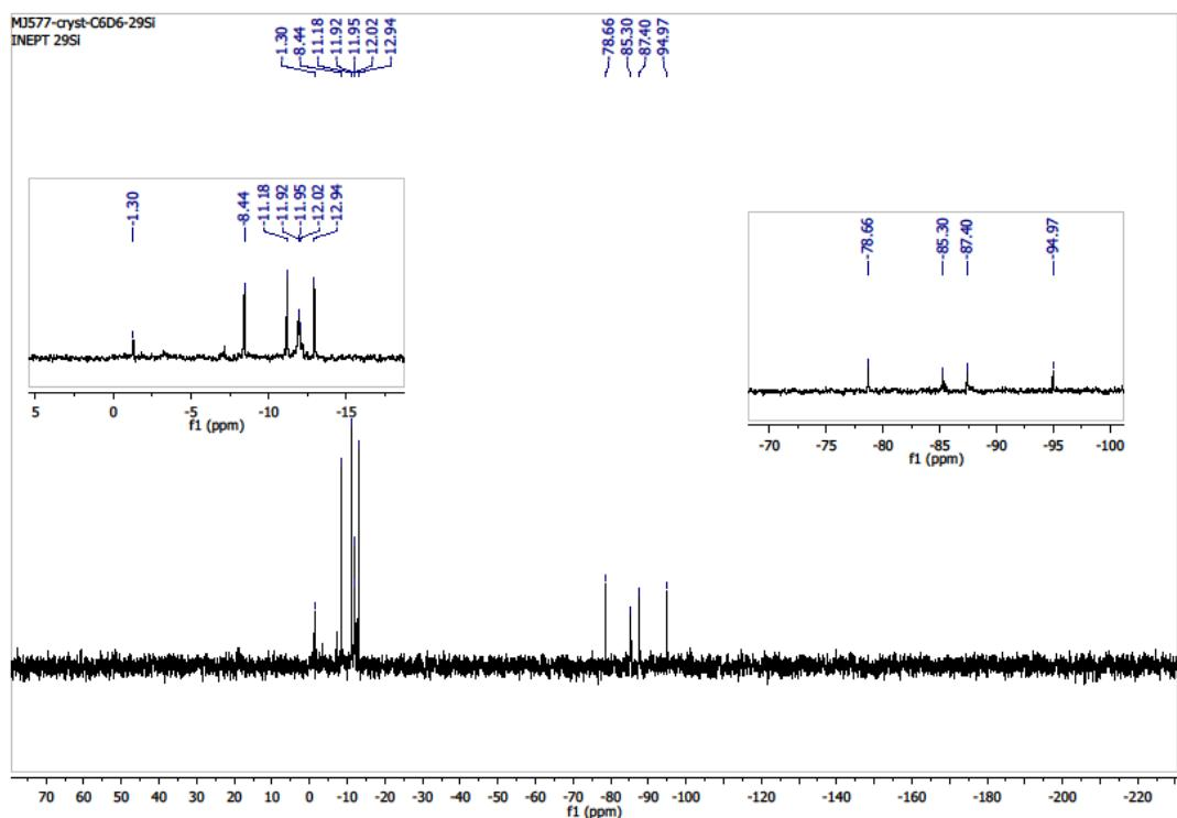
**Figure 13.**  $^{29}\text{Si}\{\text{H}\}$  INEPT NMR spectrum of **7/8a** in  $\text{C}_6\text{D}_6$
