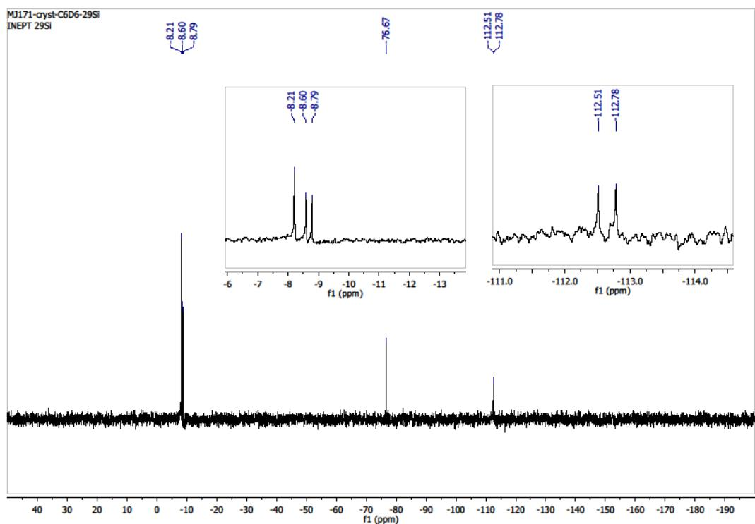
**Figure 7.**  $^{29}\text{Si}\{\text{H}\}$  INEPT NMR spectrum of **3** in C<sub>6</sub>D<sub>6</sub>
