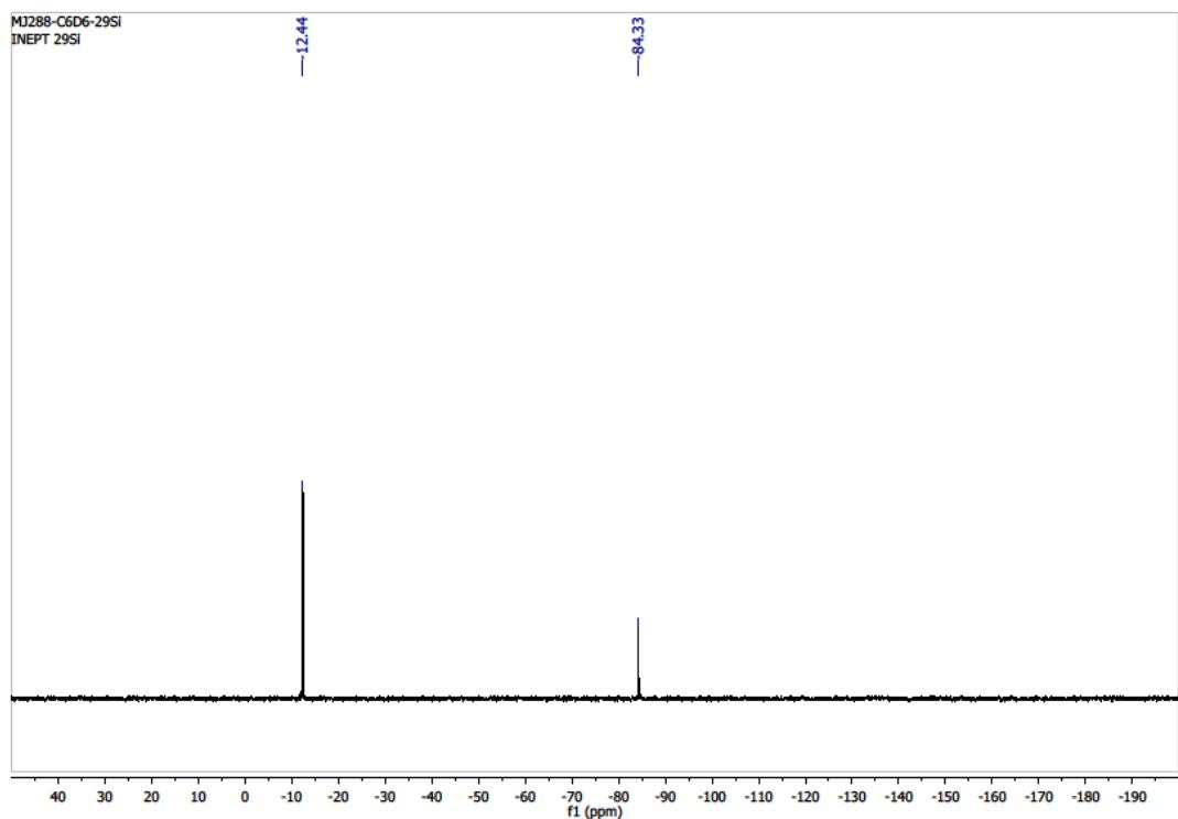
**Figure 14.**  $^{29}\text{Si}\{\text{H}\}$  INEPT NMR spectrum of **10** in  $\text{C}_6\text{D}_6$
