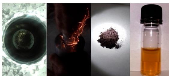
**Figure 10.** Crushing fullerenes in the presence of  $\text{Na}_2\text{O}_2$  in a stainless steel mortar and pestle caused ignition of the mixture as evidenced by the generation of bright flash. Washing of the product led to a dark brown powder, namely fullerols. Fullerols were soluble in water by mild alkaline treatment and sonication.
