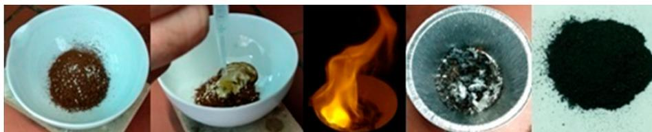
**Figure 9.** Left-to-right: instant coffee grains were mixed with  $\text{Na}_2\text{O}_2$  beads in a porcelain dish. Subsequent addition of water caused ignition of the mixture towards the formation of a crude carbon residue. After thorough washings, a fine black powder was obtained containing carbon nanosheets.
