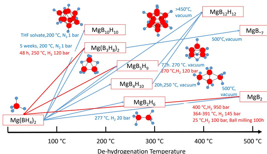
**Figure 1.** Illustration of  $\text{Mg}(\text{BH}_4)_2$  dehydrogenation reactions (blue arrows) and rehydrogenation reactions (red arrows) reported in the literature [22,34–44]. Upon further heating, these intermediate species, which are associated with (amorphous)  $\text{MgH}_2$ , form  $\text{MgB}_2$ .
