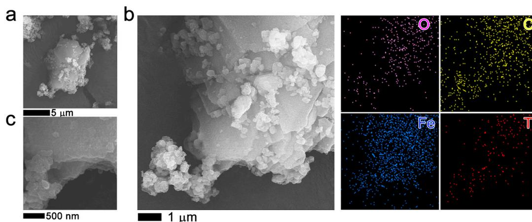
**Figure 5.** SEM images (a–c) of 2.5TiO<sub>2</sub>/MIL-100 (Fe) sample. The elemental analysis with energy dispersive X-ray spectroscopy (EDS) is plotted on the right of the SEM image.
