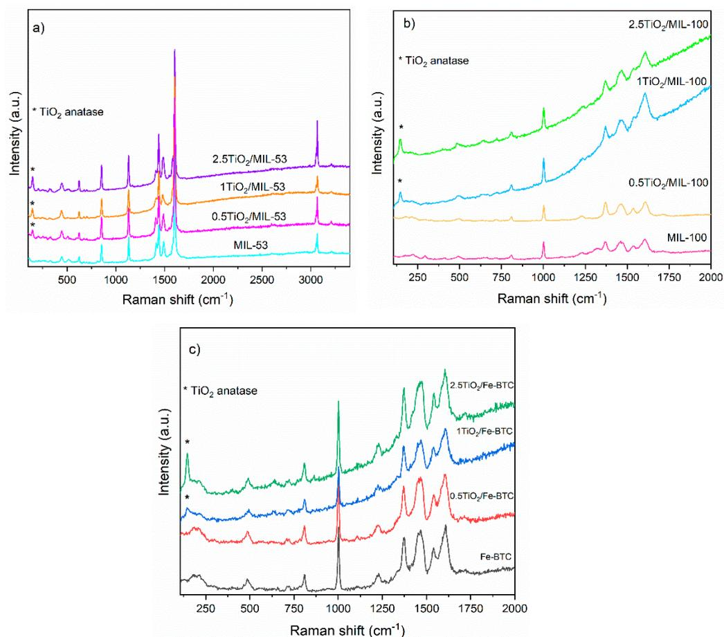
**Figure 3.** Raman spectra of (a) MIL-53 (Fe) series, (b) MIL-100 (Fe) series, and (c) Fe-BTC series.
