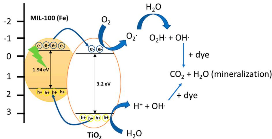
**Figure 12.** Scheme of a possible reaction mechanism in term of charge transfer in the 0.5TiO<sub>2</sub>/MIL-100 composite material.
