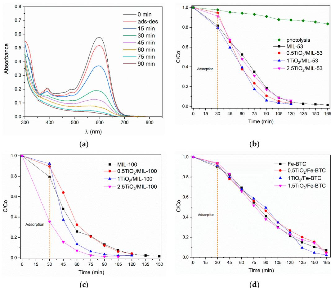
**Figure 9.** Photocatalytic activity of the Reactive Black 5 dye for the different materials. (a) UV–Vis spectra of photocatalytic degradation using MOF  $2.5\text{TiO}_2/\text{MIL-100}$ ; (b–d)  $C(t)/C_0$  concentration ratio vs. reaction time for MIL-53 (Fe), MIL-100 (Fe), and Fe-BTC, respectively.
