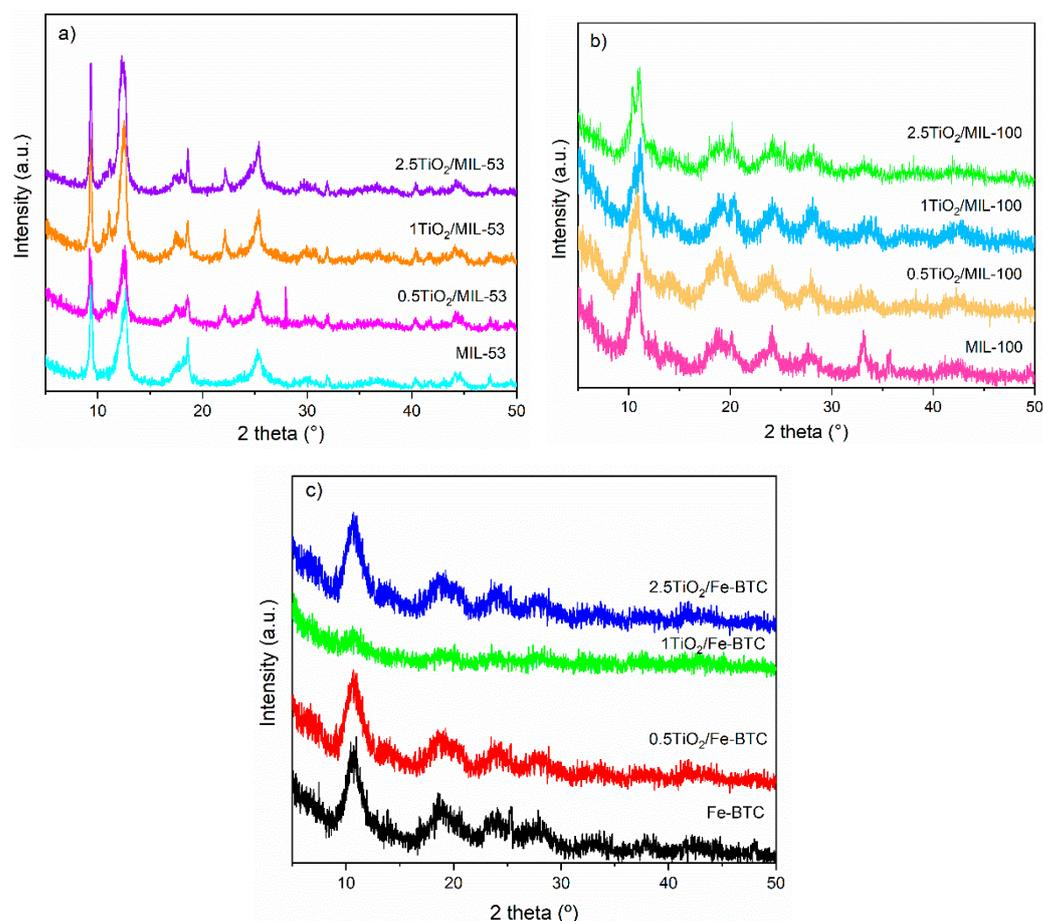
**Figure 2.** PXRD of (a) MIL-53 (Fe) series, (b) MIL-100 (Fe) series, and (c) Fe-BTC series.
