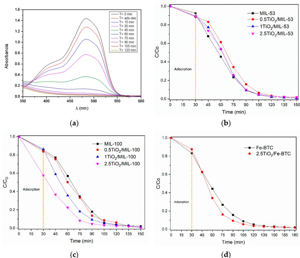
**Figure 8.** Photocatalytic activity of the Orange II dye for the different materials: (a) UV-Vis spectra obtained of the Orange II photocatalytic degradation using the  $2.5\text{TiO}_2/\text{MIL-100}$  sample; (b–d)  $C(t)/C_0$  concentration ratio vs. reaction time for MIL-53 (Fe), MIL-100 (Fe) and Fe-BTC, respectively.
