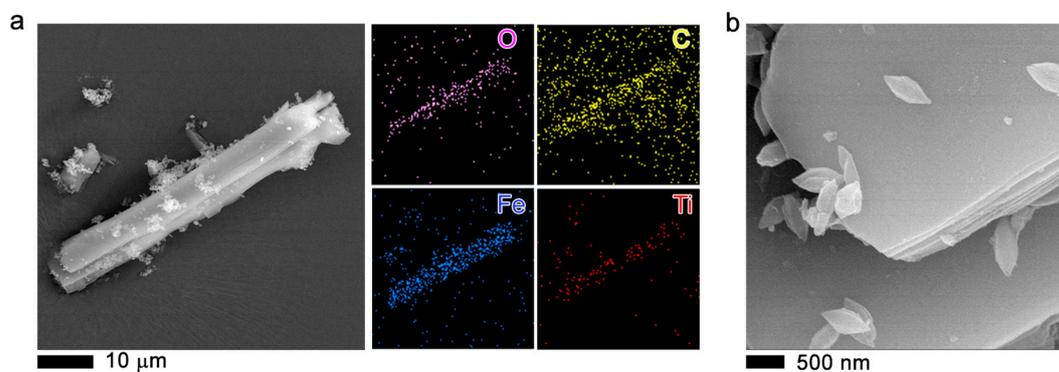
**Figure 4.** SEM images (a,b) of  $2.5\text{TiO}_2/\text{MIL-53}$  (Fe) composite material. Additionally, the elemental energy dispersive X-ray spectroscopy (EDS) maps are plotted on the right of the panel (a).
