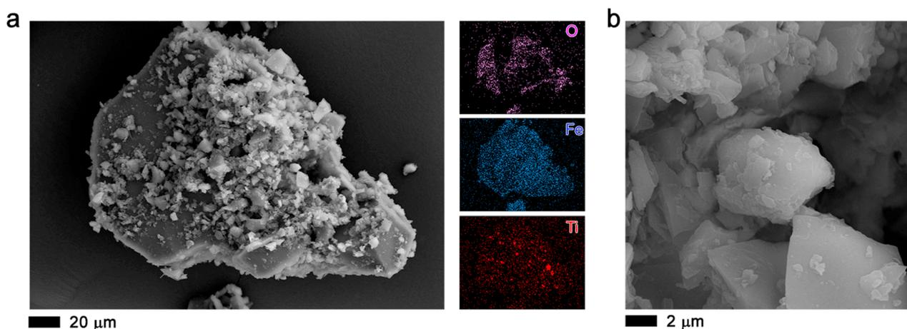
**Figure 6.** MOF Fe-BTC, SEM images (a,b). The elemental analysis with energy dispersive X-ray spectroscopy (EDS) is plotted on the right of panel (b).
