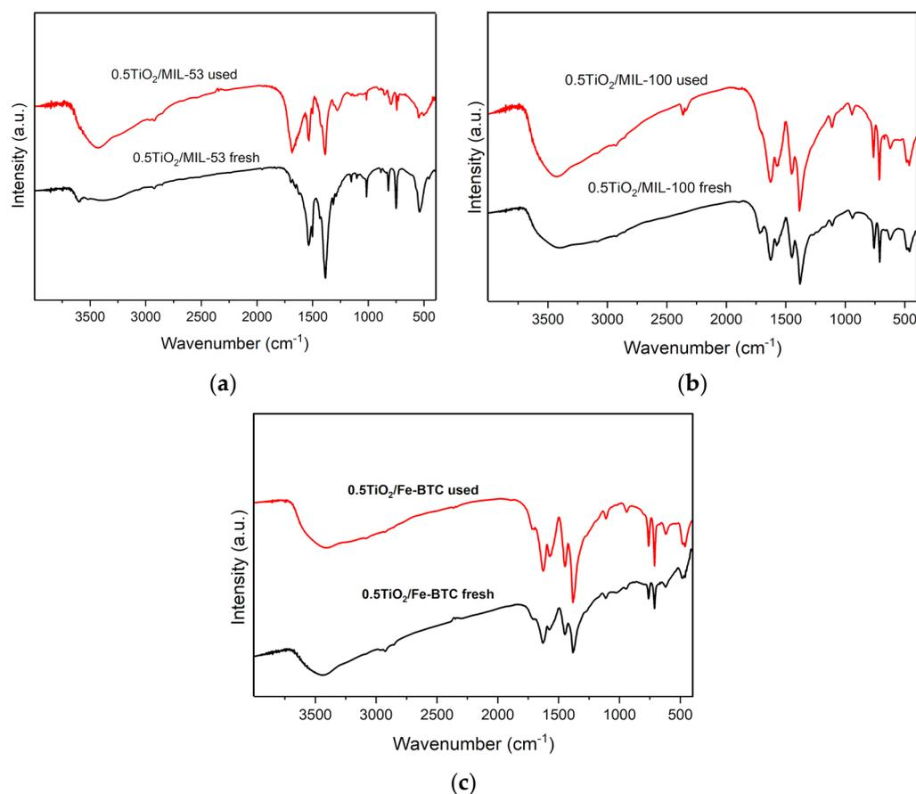
**Figure 10.** FTIR spectra of the fresh and used composite materials of (a) 0.5TiO<sub>2</sub>/Fe-BTC, (b) 0.5TiO<sub>2</sub>/MIL-53, and (c) 0.5TiO<sub>2</sub>/MIL-100.
