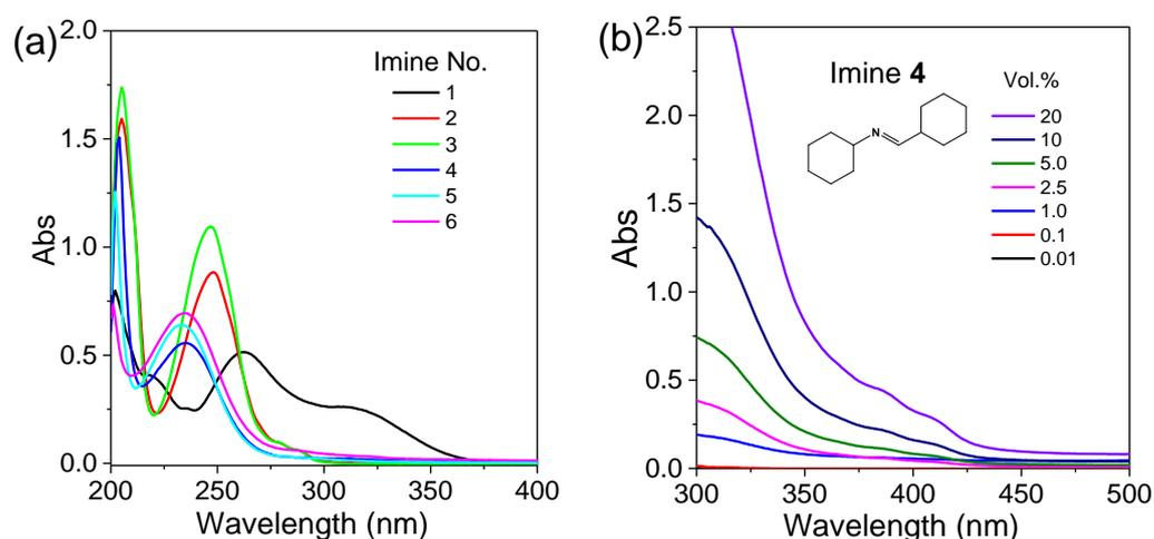
**Figure 1.** (a) UV-vis spectra of imines 1–6 ethanol solutions (2–6: 0.01 vol.%, 1: 0.0001 mol L<sup>-1</sup>). (b) UV-vis spectra of imine 4 ethanol solutions with different concentrations.
