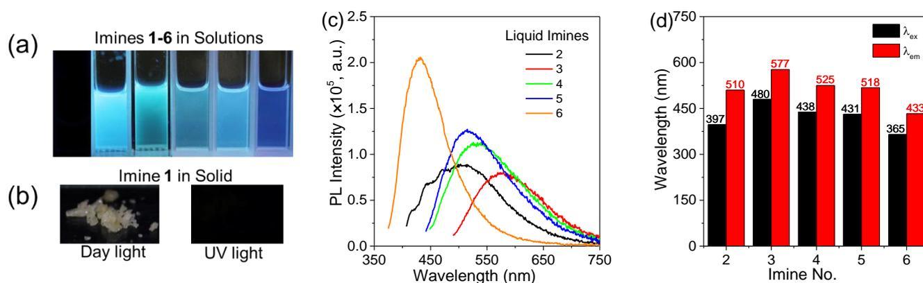
**Figure 2.** (a) Photographs of imines 2–6 ethanol solutions (5 vol.%) under 365 nm UV light, and (b) photographs of imine 1 solid powders under daylight and 365 nm UV light. (c) Fluorescence emission spectra of pure imines 2–6 in liquid state, and (d) their maximum excitation wavelength (black) and maximum emission wavelength (red).
