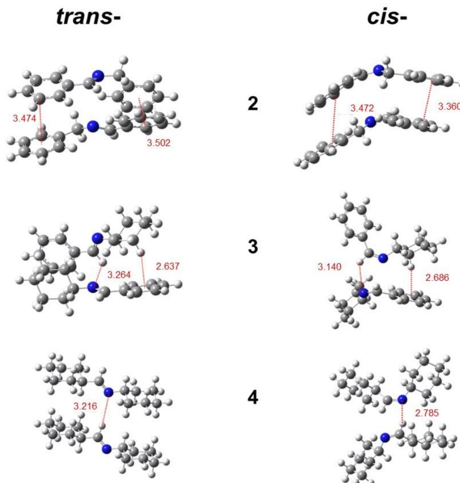
**Figure 6.** Optimized conformations of the dimers of imines **2**, **3**, and **4** in *trans*- and *cis*-configurations.
