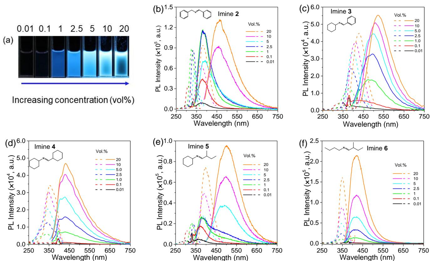
**Figure 3.** (a) Photographs of imine 6 ethanol solutions with different concentrations under 365 nm UV light (from left to right, Vol.% = 0.01%, 0.1%, 1.0%, 2.5%, 5%, 10%, 20%). (b–f) Fluorescence excitation spectra (dashed line) and emission spectra (solid line) of imines 2–6 ethanol solutions with different concentrations.
