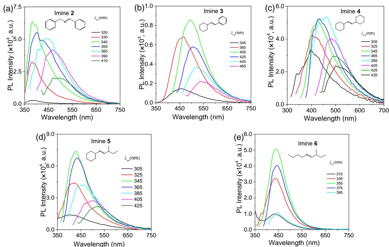
**Figure 4.** Fluorescence emission spectra of imines 2–6 ethanol solutions (5 vol.%) at different excitation wavelengths. (a–e): imines 2–6, respectively.
