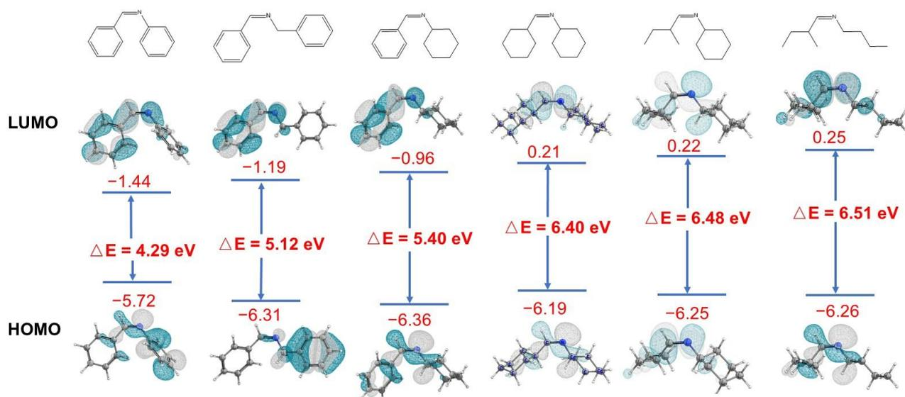
**Figure 5.** HOMO and LUMO orbitals of different imines in *cis*-configuration.
