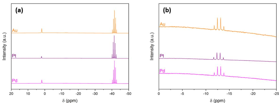
**Figure 2.**  $^{11}\text{B}$  NMR spectra of the aqueous alkaline (0.1 M NaOH) solution of  $\text{BH}_4^-$  (0.66 M; i.e., 50 mg  $\text{NaBH}_4$  in 2 mL) upon  $\text{H}_2$  evolution catalyzed by Pd, Pt, or Au at 30 °C. (a) Range between  $\delta +20$  and  $\delta -50$  ppm. (b) Focus on the range between  $\delta 0$  and  $-25$  ppm.
