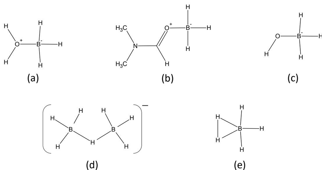
**Figure 5.** Possible  $\text{BH}_3$  intermediates showing a quartet in  $^{11}\text{B}$  NMR: (a)  $\text{H}_2\text{O}\cdot\text{BH}_3$ , (b)  $\text{DMF}\cdot\text{BH}_3$ , (c)  $\text{BH}_3\text{OH}^-$ , (d)  $\text{B}_2\text{H}_7^-$ , and (e)  $\text{BH}_3(\text{H}_2)$ .
