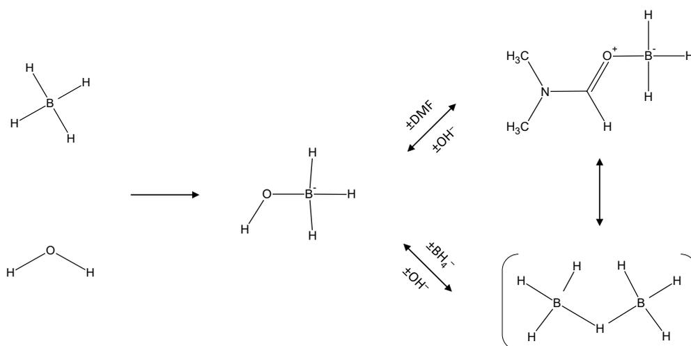
**Figure 6.** Mechanistic sequence illustrating the formation of the identified BH<sub>3</sub>-based intermediates BH<sub>3</sub>OH<sup>-</sup>, DMF·BH<sub>3</sub>, and B<sub>2</sub>H<sub>7</sub><sup>-</sup>.
