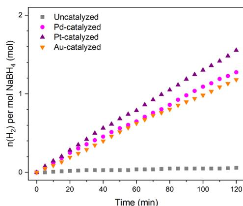
**Figure 1.**  $\text{H}_2$  evolution curve for the hydrolysis of 2 mL of an aqueous alkaline (0.1 M NaOH) solution of  $\text{BH}_4^-$  (0.66 M; i.e., 50 mg  $\text{NaBH}_4$  in 2 mL) catalyzed by 16.1 mg of Pd, 14.5 mg of Pt, or 14.3 mg of Au at 30 °C. The  $\text{H}_2$  evolution curve for the uncatalyzed hydrolysis test is also shown. The  $y$ -axis has been limited to the range 0–2 for clarity.
