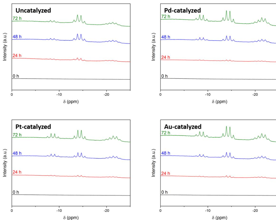
**Figure 3.**  $^{11}\text{B}$  NMR spectra of the 10 mL DMF solutions of  $\text{BH}_4^-$  (1.32 M) hydrolyzed by 7.6 mL of alkaline (0.1 M NaOH), uncatalyzed or catalyzed by Pd, Pt, or Au after 0, 24, 48 and 72 h. These spectra focus on the range between  $\delta$  0 ppm and  $\delta$  -25 ppm to show the signals at  $\delta < 0$  ppm.
