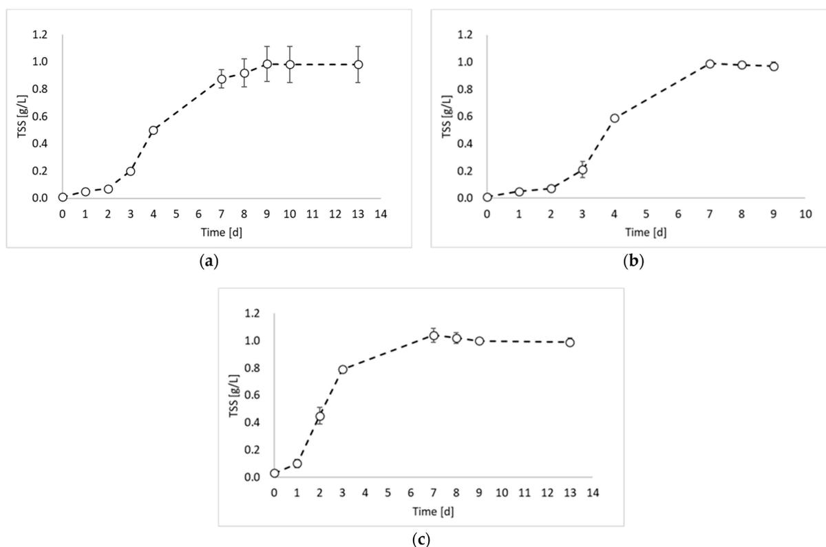
**Figure 1.** Total suspended solids (TSSs) concentration over time obtained during: (a) biomass growth, (b) inoculum production, and (c) hydrogen production tests.
