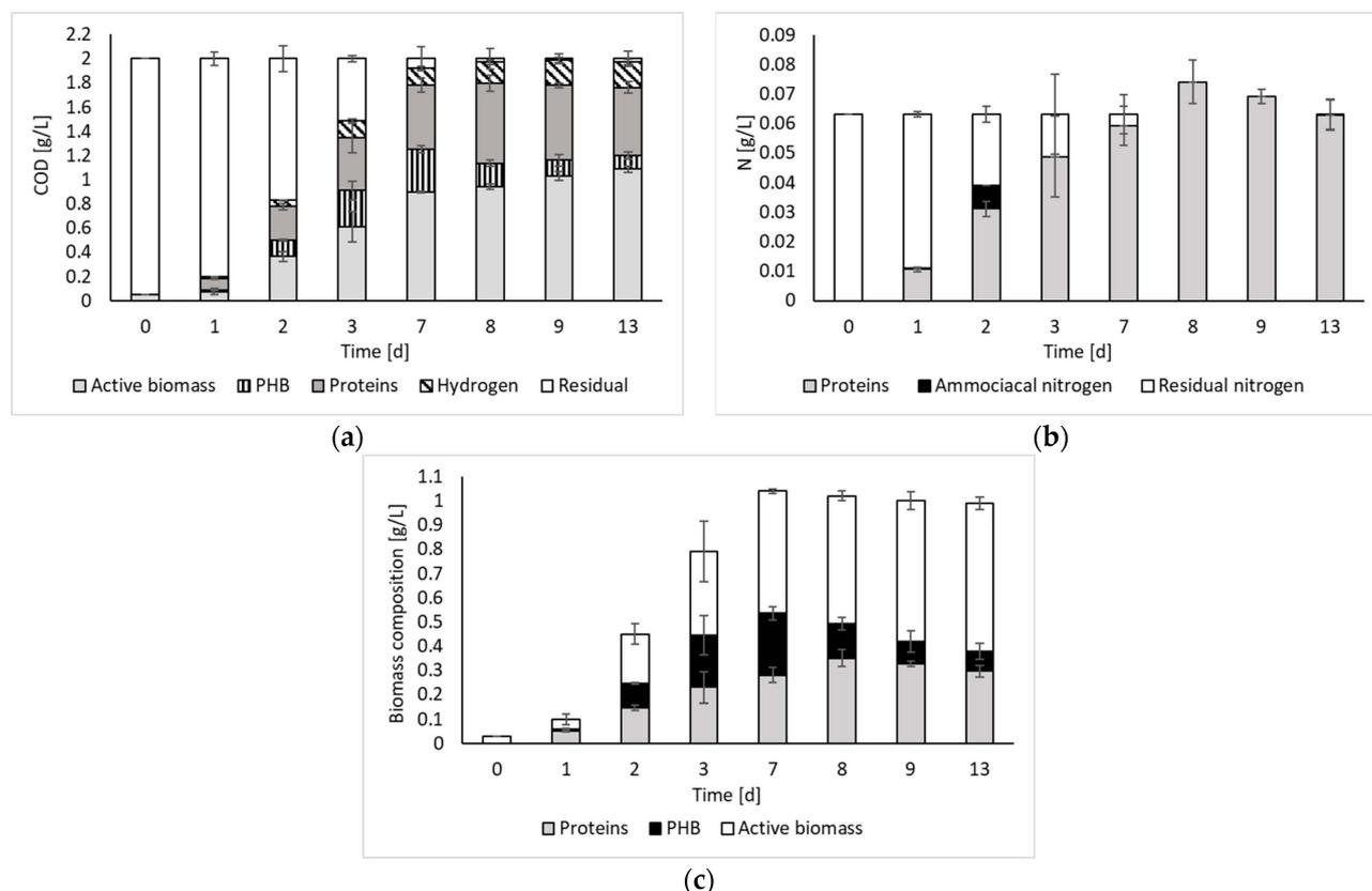
**Figure 3.** COD (a) and nitrogen (b) balances, and biomass composition (c) over time.
