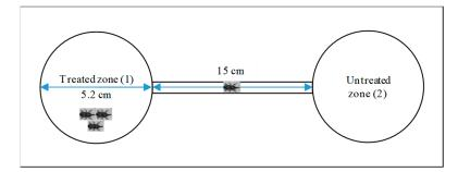
**Figure 7.** Modified tunnel-type device to measure the repellent effect on maize weevils (sketch made by authors).
