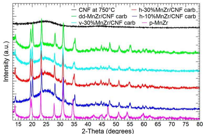
**Figure 2.** XRPD patterns of CNFs, pristine  $\text{Na}_3\text{MnZr}(\text{PO}_4)_3$  powder, and self-standing cathodes.
