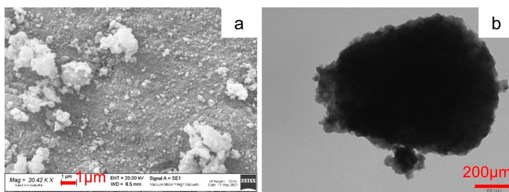
**Figure 4.** SEM and TEM images of  $\text{Na}_3\text{MnZr}(\text{PO}_4)_3$  powder: (a) 20.42 kX and (b) 100 kX.
