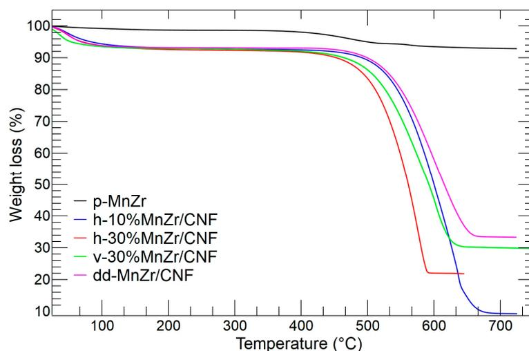
**Figure 11.** TGA analysis of p-MnZr (black), h-10%MnZr/CNF (blue), h-30%MnZr/CNF (red) v-30%MnZr/CNF (green), and dd-MnZr/CNF (purple) samples.
