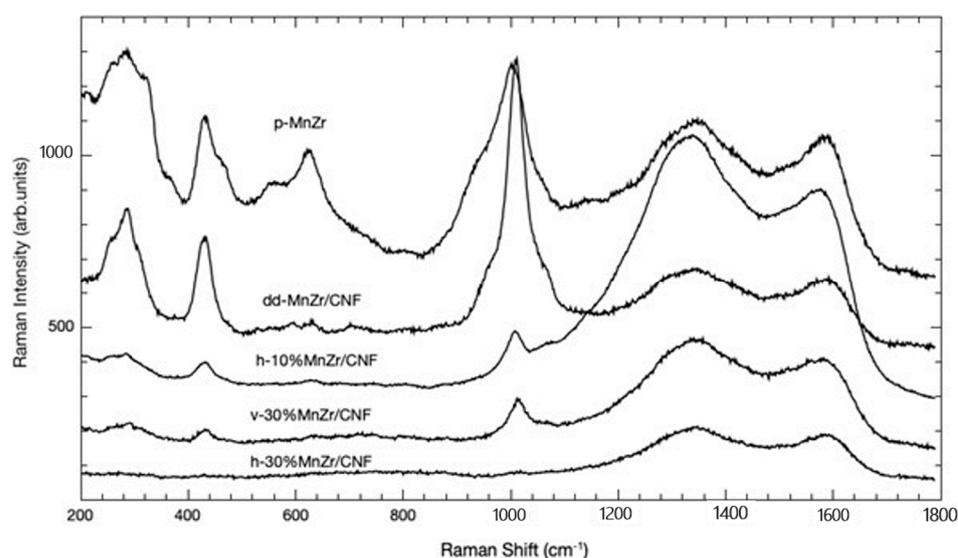
**Figure 3.** Raman spectra of p-MnZr, h-10%MnZr/CNF, h-30%MnZr/CNF, v-30%MnZr/CNF, and dd-MnZr/CNF samples.
