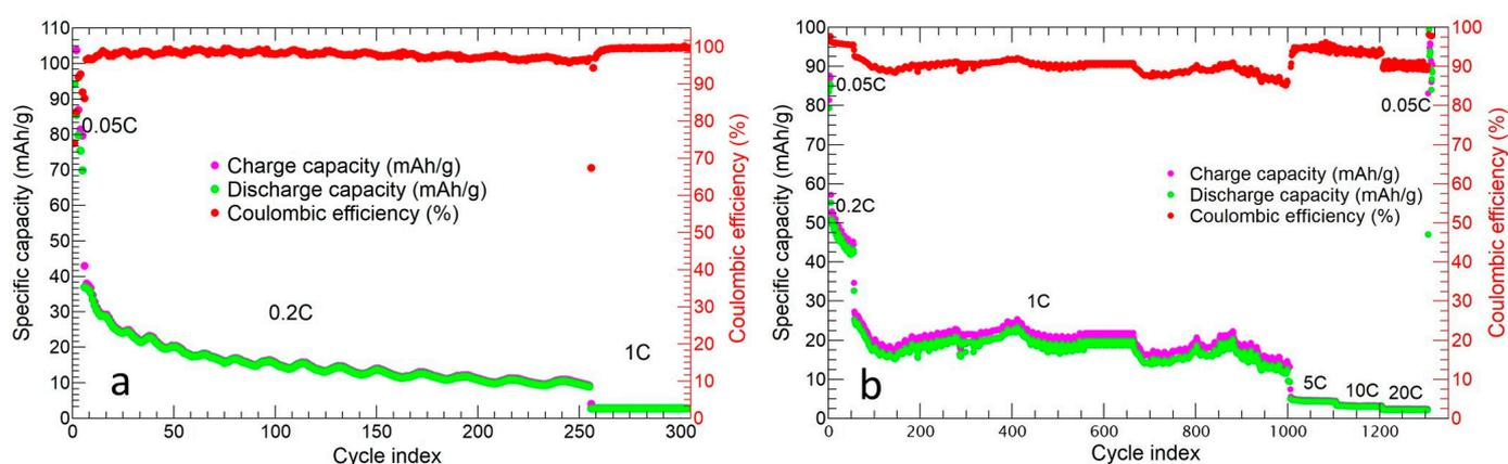
**Figure 13.** Cycling performance of (a) p-MnZr slurry electrode and (b) v-30%MnZr/CNF self-standing cathode.
