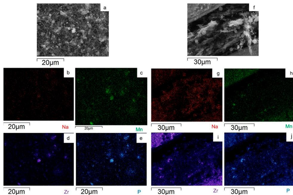
**Figure 7.** SEM image and EDS maps of the different elements for the h-10%MnZr/CNF (a–e) surface and (f–j) its cross-section.
