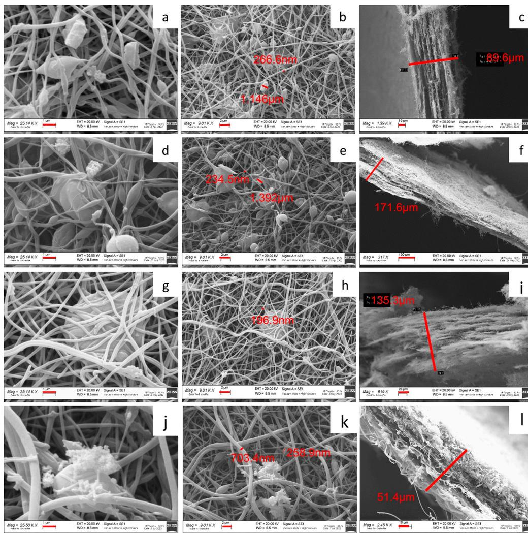
**Figure 5.** SEM images of h-10%MnZr/CNF (a,b) surface and (c) cross-section; h-30%MnZr/CNF (d,e) surface and (f) cross-section; v-30%MnZr/CNF (g,h) surface and (i) cross-section; and dd-MnZr/CNF (j,k) surface and (l) cross-section.
