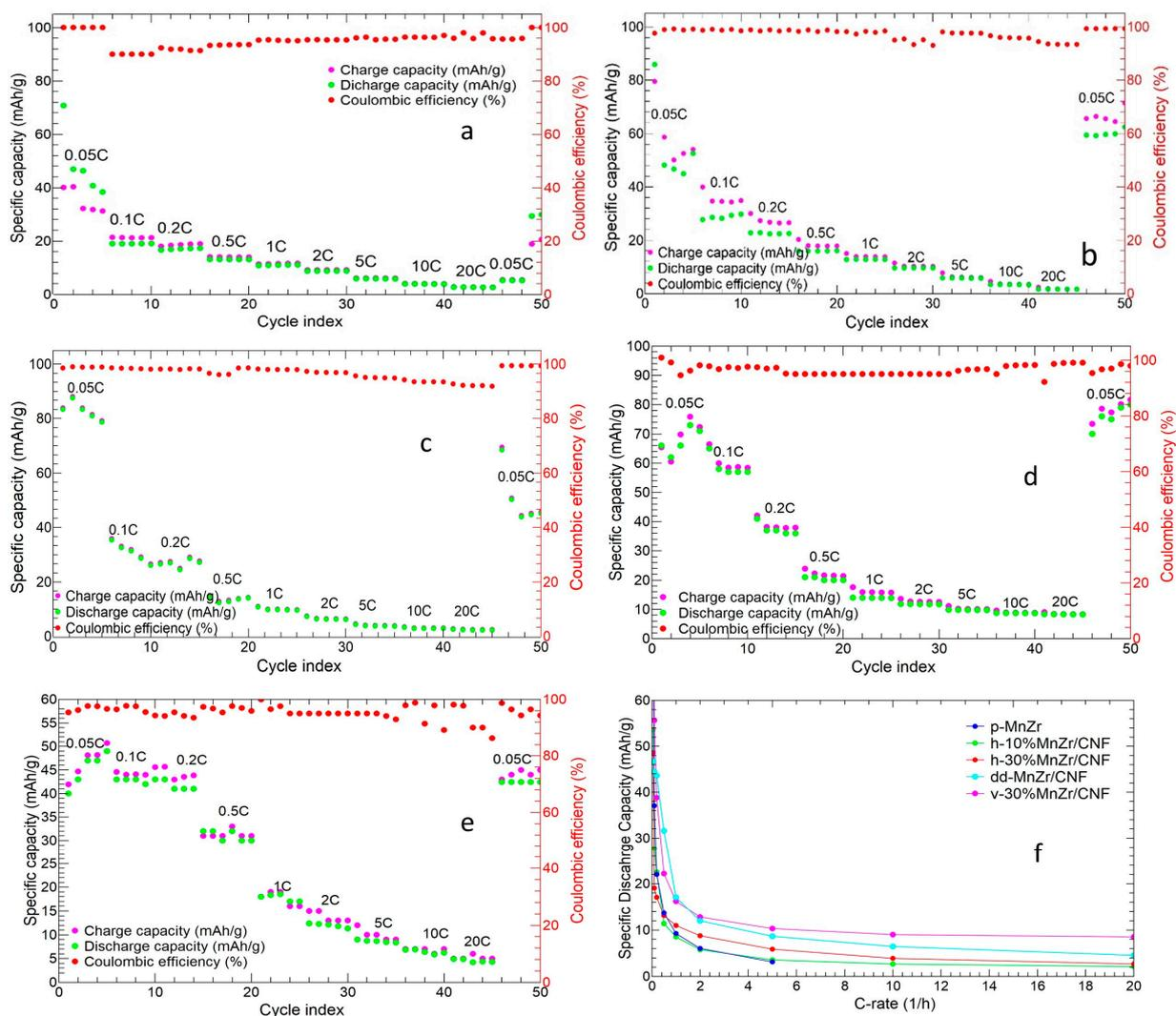
**Figure 12.** Charge/discharge cycles at different C-rates of (a) p-MnZr, (b) h-10%MnZr/CNF, (c) h-30%MnZr/CNF, (d) v-30%MnZr/CNF, and (e) dd-MnZr/CNF; (f) comparison of average discharge capacity values for all the samples at different C-rates.
