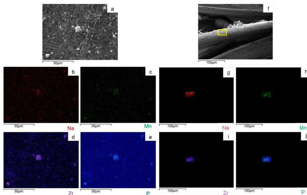
**Figure 9.** SEM image and EDS maps of the different elements for the v-30%MnZr/CNF (a–e) surface and (f–j) its cross-section. The yellow frame indicates the mapped portion.
