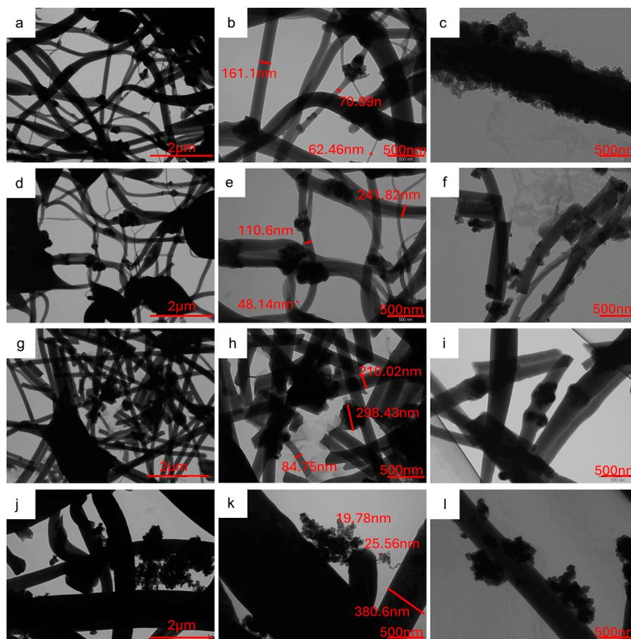
**Figure 6.** TEM images at different magnifications (20 kX e 50 kX) of (a–c) h-10%MnZr/CNF, (d–f) h-30%MnZr/CNF, (g–i) v-30%MnZr/CNF, and (j–l) dd-MnZr/CNF samples.
