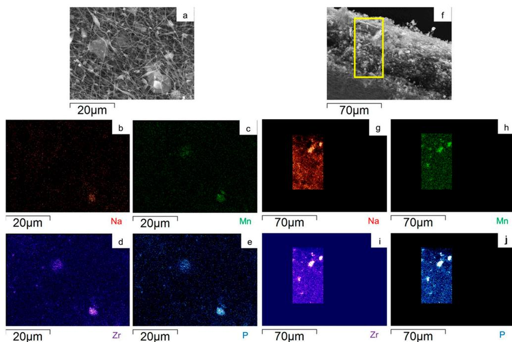
**Figure 8.** SEM image and EDS maps of the different elements for the h-30%MnZr/CNF (a–e) surface and (f–j) its cross-section. The yellow frame indicates the mapped portion.
