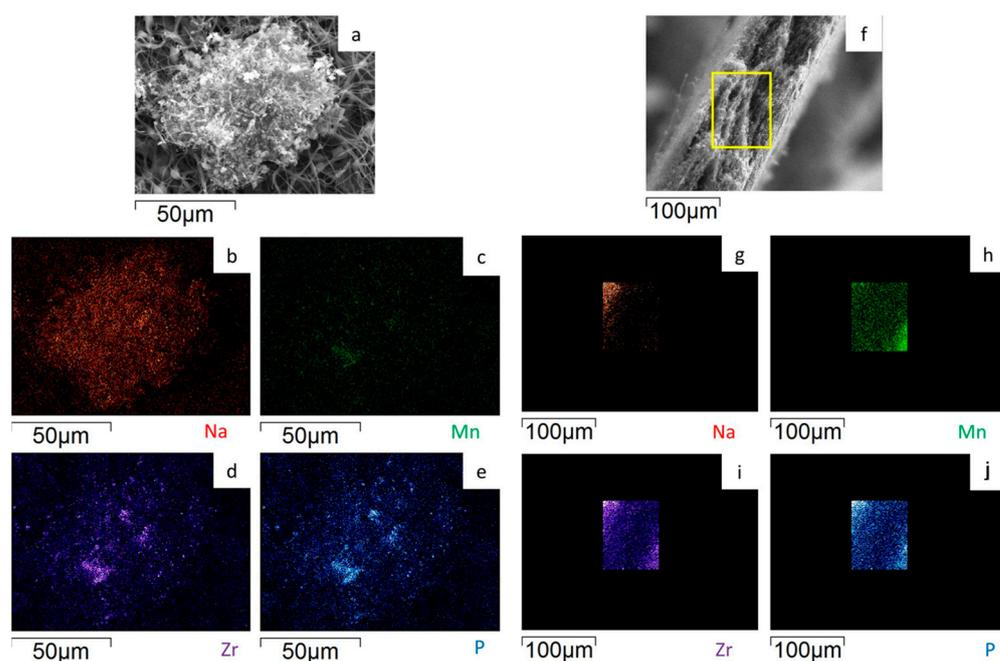
**Figure 10.** SEM image and EDS maps of the different elements for the dd-MnZr/CNF (a–e) surface and (f–j) its cross-section. The yellow frame indicates the mapped portion.
