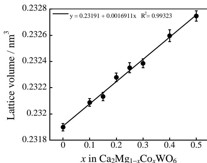
**Figure 4.** Composition dependence of the lattice volume of the  $\text{Ca}_2\text{Mg}_{1-x}\text{Co}_x\text{WO}_6$  ( $0 \leq x \leq 0.50$ ) samples.
