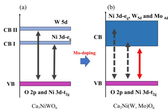
**Figure 1.** Schematic illustration of band structure for (a)  $\text{Ca}_2\text{NiWO}_6$  and (b)  $\text{Ca}_2\text{Ni}(\text{W}, \text{Mo})\text{O}_6$ . The black arrows indicate the band gap energy of the host compound, whereas the red arrows indicate the band gap energy of the Mo-doped compound.
