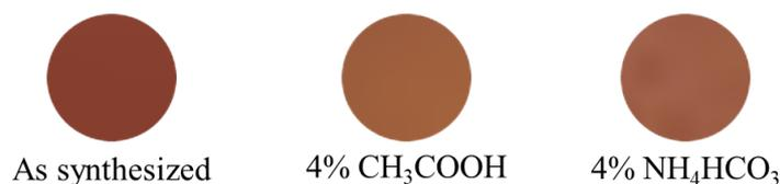
**Figure 14.** Photographs of Ca<sub>2</sub>Mg<sub>0.85</sub>Co<sub>0.15</sub>W<sub>0.50</sub>Mo<sub>0.50</sub>O<sub>6</sub> samples before and after the chemical stability test.
