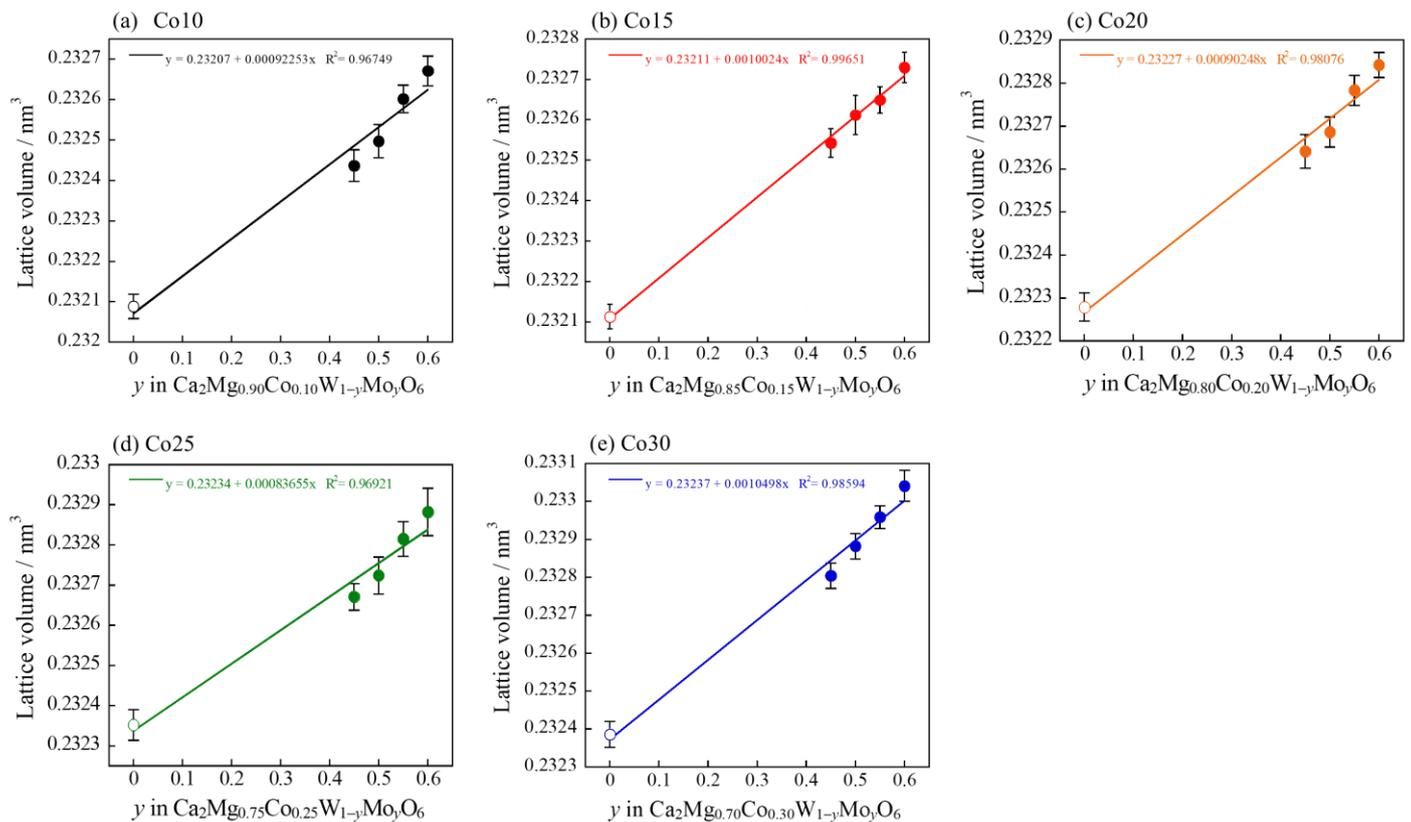
**Figure 8.** Composition dependence of the lattice volume of the  $\text{Co}_a\text{Mo}_b$  samples: (a)  $a = 10$ ; (b)  $a = 15$ ; (c)  $a = 20$ ; (d)  $a = 25$ ; and (e)  $a = 30$ .
