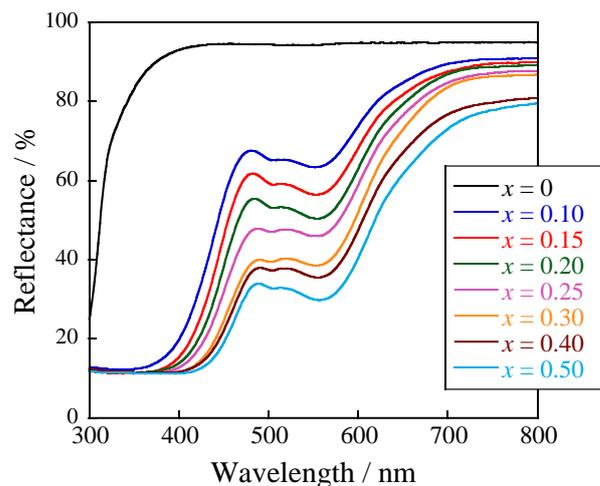
**Figure 5.** UV-vis reflectance spectra of the  $\text{Ca}_2\text{Mg}_{1-x}\text{Co}_x\text{WO}_6$  ( $0 \leq x \leq 0.50$ ) samples.
