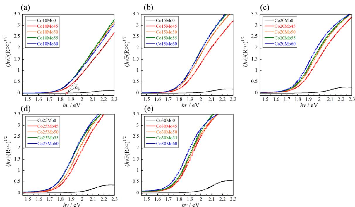
**Figure 11.** Tauc plot of the CoaMob samples: (a)  $a = 10$ ; (b)  $a = 15$ ; (c)  $a = 20$ ; (d)  $a = 25$ ; and (e)  $a = 30$ .
