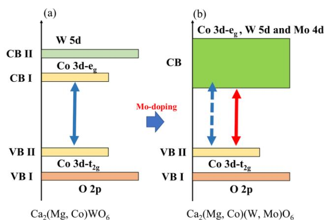
**Figure 10.** Schematic illustration of band structure for (a)  $\text{Ca}_2(\text{Mg, Co})\text{WO}_6$  and (b)  $\text{Ca}_2(\text{Mg, Co})(\text{W, Mo})\text{O}_6$ . The blue arrows indicate the band gap energy of the host compound, whereas the red arrows indicate the band gap energy of the Mo-doped compound.
