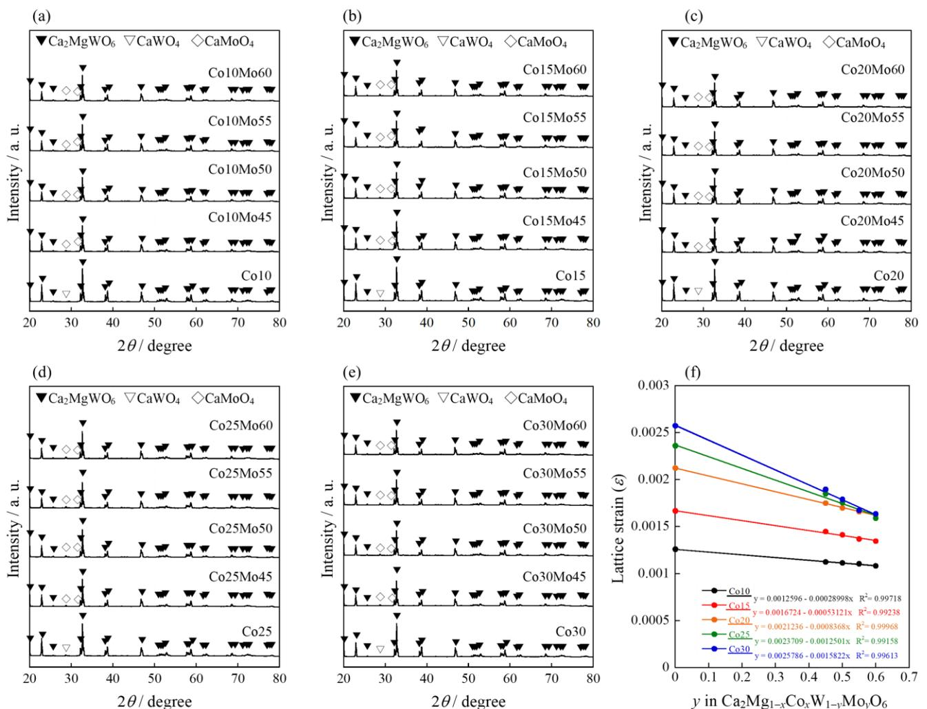
**Figure 7.** XRD patterns of the *CoaMob* samples: (a) *a* = 10; (b) *a* = 15; (c) *a* = 20; (d) *a* = 25; and (e) *a* = 30. (f) Composition dependence of lattice strain ( $\epsilon$ ) for *CoaMob* calculated by W–H analysis.
