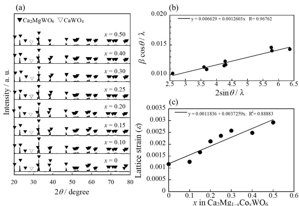
**Figure 2.** (a) XRD pattern of the  $\text{Ca}_2\text{Mg}_{1-x}\text{Co}_x\text{WO}_6$  ( $0 \leq x \leq 0.50$ ) samples; (b) Williamson-Hall (W-H) plot of  $\text{Ca}_2\text{MgWO}_6$ ; and (c) composition dependence of lattice strain ( $\epsilon$ ) calculated by W-H analysis.
