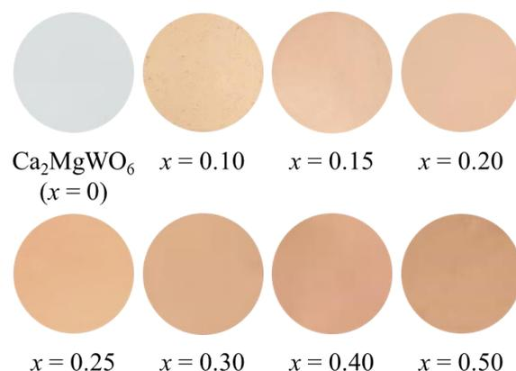
**Figure 6.** Photographs of the  $\text{Ca}_2\text{Mg}_{1-x}\text{Co}_x\text{WO}_6$  ( $0 \leq x \leq 0.50$ ) powder samples.
