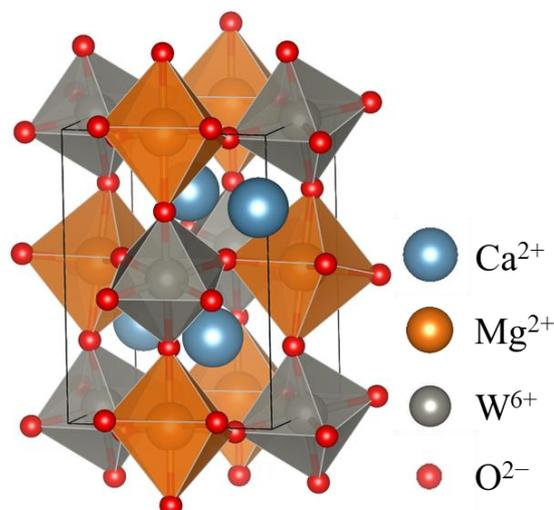
**Figure 3.** Crystal structure of double-perovskite  $\text{Ca}_2\text{MgWO}_6$ ; Ca: blue, Mg: orange, W: gray, O: red.
