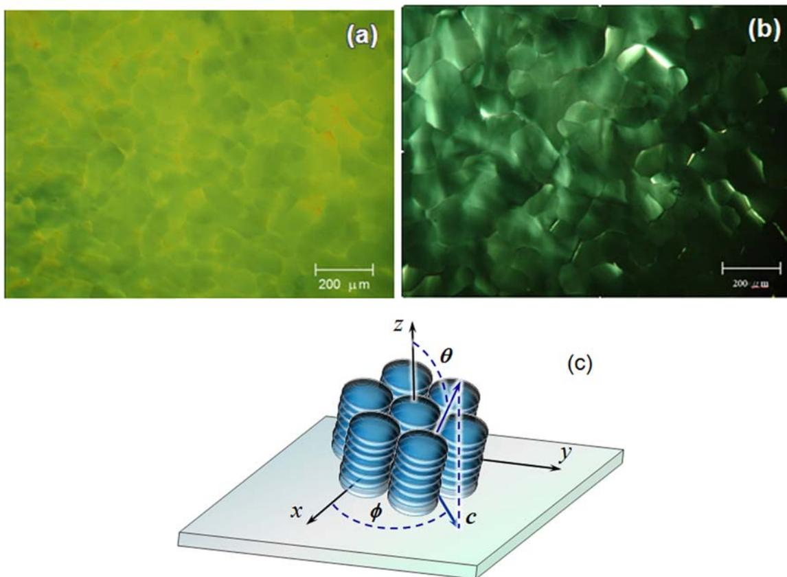
**Figure 7.** Light transmittance of LC10 layers sandwiched by substrates that were O<sub>2</sub> plasma bombarded for different period. Prolongation of the exposure period of the substrates to the plasma can cause a decrease in light transmittance of the DLC samples.
