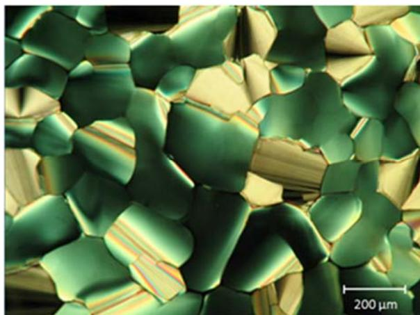
**Figure 4.** LC10 in a confined cell made using glass plates. The sample was cooled down to 120 °C from an elevated temperature at a cooling rate of 0.1 °C/min. The pattern reflects a hexagonal symmetry of the columnar structure with the face-on molecular anchoring.
