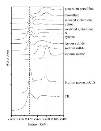
**Figure 4.** Comparison of sulfur K-edge XANES in *Halothiobacillus* HT1 biofilm (CK), *Halothiobacillus* HT1 biofilm reacted with CuS and reference compounds.
