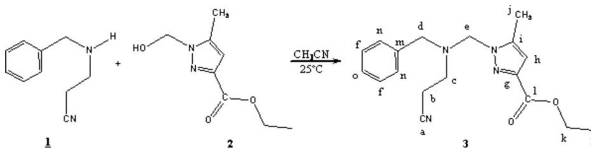
A mixture of 3-(benzylamino)propionitrile **1** [3] (1g, 6.25mmol) and 1-hydroxymethyl-5-methyl-1H-pyrazole-3-carboxylic acid ethyl ester **2** [4] (1.15g, 6.25 mmol) in 20 ml of acetonitrile was stirred at room temperature for four days, then the mixture was dried with Na<sub>2</sub>SO<sub>4</sub> and filtered. The solvent was evaporated under reduced pressure. The product **3** obtained with an 81% yield as yellow oil.
