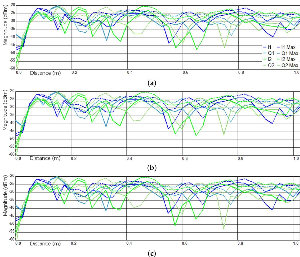
**Figure A3.** Frequency domain data plots: (a,b) for no-insect conditions, (c) an insect in H2 (notice the higher amplitudes). Vertical axes are the magnitude levels in dBm; horizontal axes are the distances in meters.
