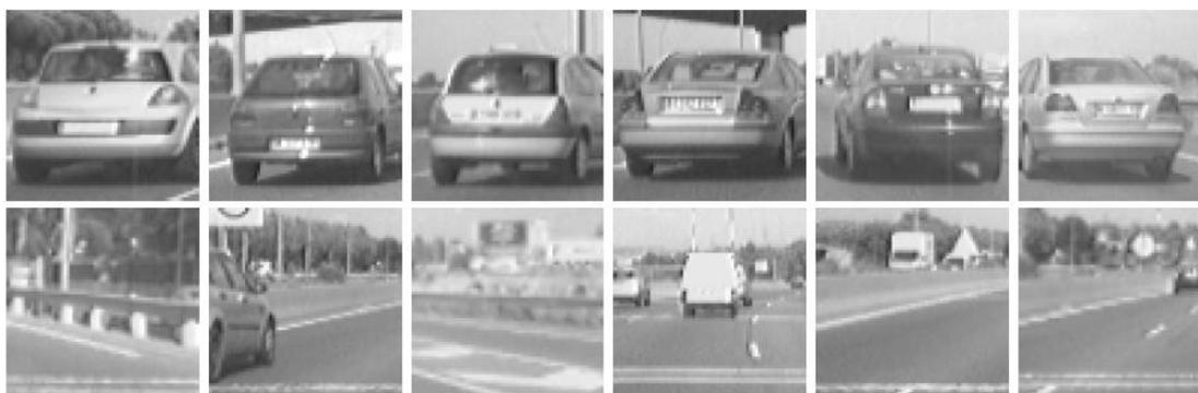
**Figure 11.** Rear data set. Upper row: positive samples (vehicles); Lower row: negative samples.
