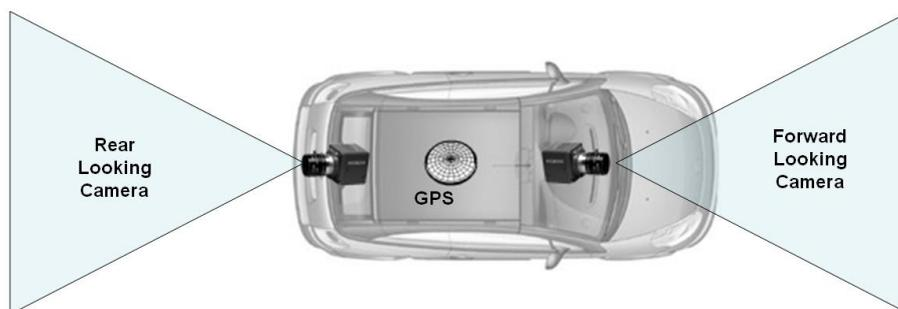
Each individual vehicle detection system provides information about the number of detected vehicles and both their relative position and speed. These results are combined with the GPS measurements and the data provided by the CAN bus (vehicle speed) in order to provide globally referenced traffic information. Note that for vehicles without CAN bus interface, the vehicle speed can be computed from GPS measurements. This scheme is described in Figure 2.
