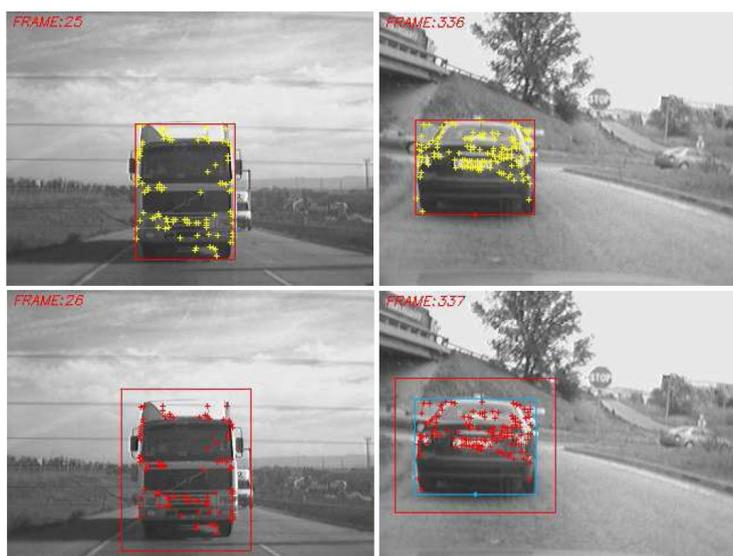
Tracking is implemented using Kalman filtering techniques [10]. For this purpose, a dynamic state model and a measurement model must be defined. The proposed dynamic state model is simple. Let us consider the state vector  $x_n$ , defined as follows:
