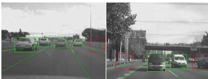
After detecting consecutively an object classified as vehicle a predefined number of times (empirically set to 3 in this work), data association and tracking stages are triggered. The data association problem is addressed by using feature matching techniques. Harris features are detected and matched between two consecutive frames, as depicted in Figure 13.
