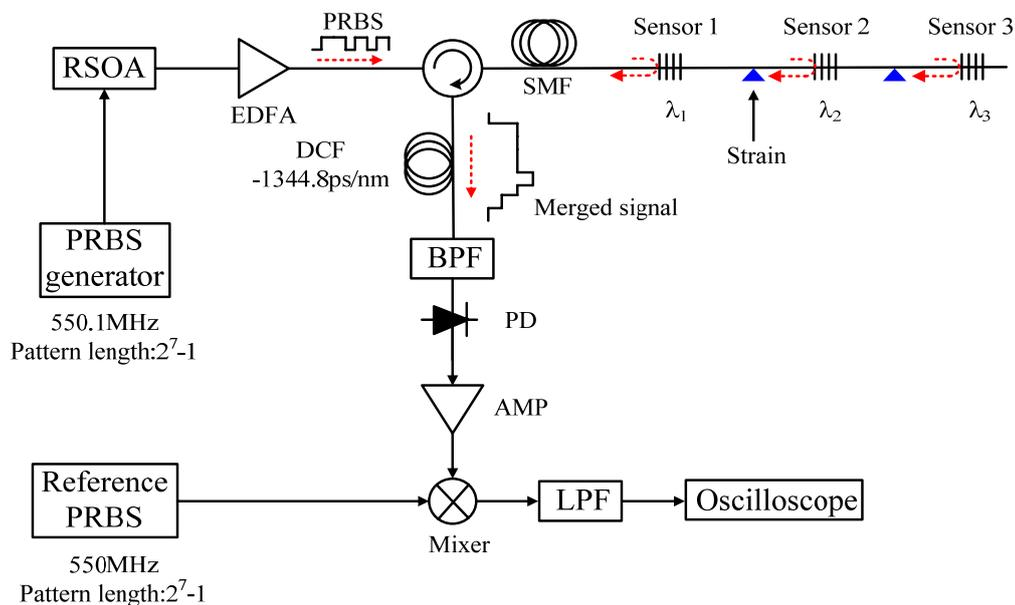
RSOA: reflective semiconductor optical amplifier, EDFA: erbium doped fiber amplifier, PRBS: pseudo random binary sequence, SMF: single mode fiber, DCF: dispersion compensation fiber, BPF: bandpass filter, PD: photodetector, AMP: amplifier, LPF: low pass filter
