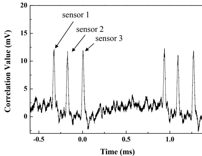
**Figure 4.** (a) Measured autocorrelation pulses. (b) Improved autocorrelation traces after using the BPF.
