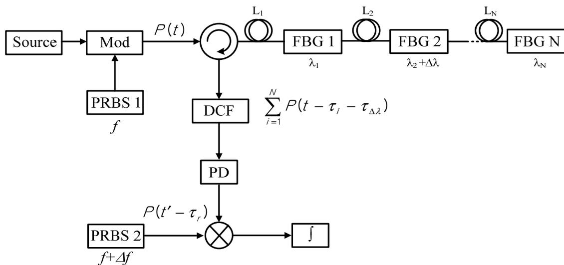
Mod: modulator, FBG: fiber Bragg grating, DCF: dispersion compensation fiber (wavelength to time conversion module), PRBS: pseudo random binary sequence, PD: photodetector
