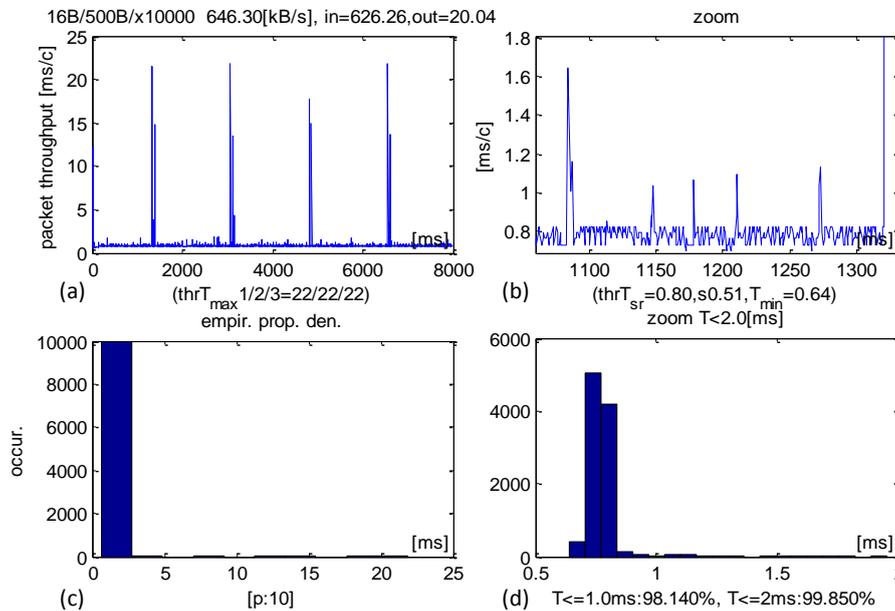
Packets of 2500 B transacted on average in 3.52 ms. The SD parameter equalled 0.79 ms. 99.36% transactions executed within 4 ms and 99.82% within than 5 ms. A detailed analysis (Figure 7) shows very long delays of 60 ms, as a result of pre-emption by the OS. Similarly, high values (50–60 ms) were also observed in other experiments. The average sensor data stream received was 714 KB/s.
