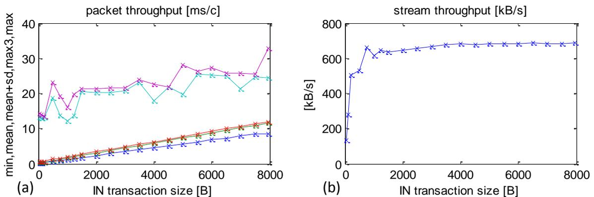
In terms of the throughput of the sensor data stream received the dual-thread architecture was slightly outperformed by the single-thread solution. The largest packets achieved a throughput of 686 KB/s.
