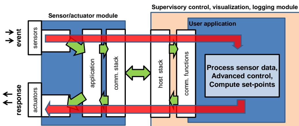
In typical acquisition/control applications packets sent out from supervisory control module (OUT) are relatively short. They contain coded requests for the retrieval of sensors data and such a packet contains only between 10 and 20 bytes. The packets can also contain control data computed in the tablet and intended for the DA, PWM converters or digital output lines.
