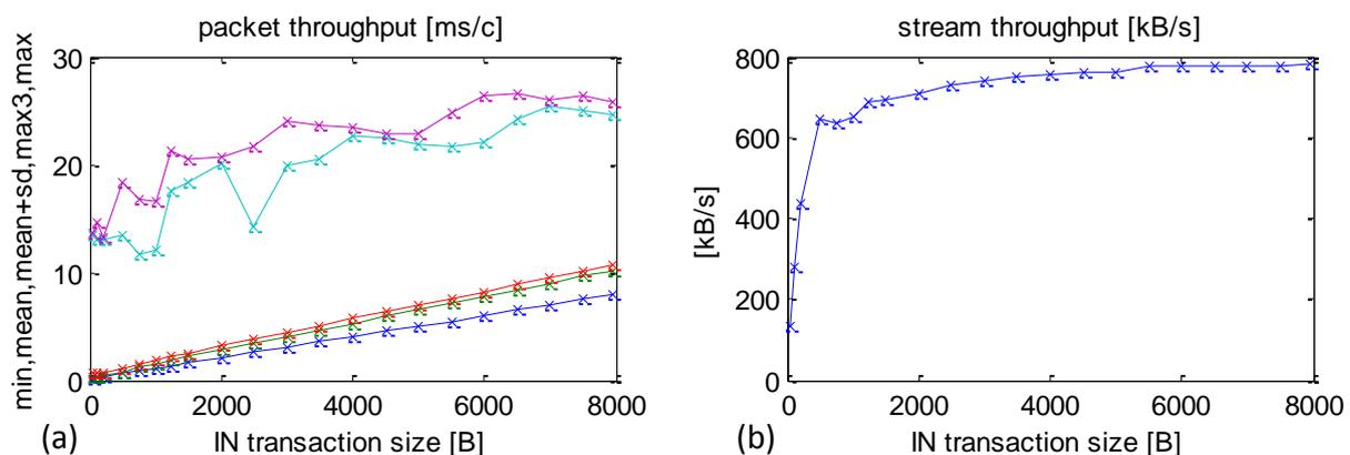
This optimisation variant produced a further CCLT reduction in the worst cases, especially with small packets (Figure 12a maximum CCLT cyan curve). Transactions with packet sizes 48 B, 100 B, 200 B (IN) never exceeded 15 ms. This is a very important result for specialised control applications, because it determines the maximum timing of a closed control loop.
