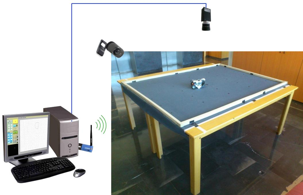
The server is implemented in the LabVIEW programming language. This graphical language was selected because it allows direct connection with the LEGO NXT robot and gives advanced image processing capabilities that are used to compute the robot position.
