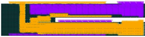
Therefore, two groups of nodes are created. Each electrode is defined by 2,317 elements that are translated into 6,390 nodes. An independent voltage source links one node from each of the two groups together implemented by using the element CIRCU94. One group is defined as the loaded electrode such that a symmetric sinusoidal voltage wave is supplied to it, while the other electrode is grounded.
