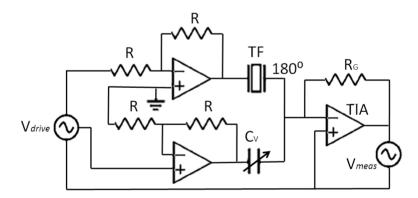
As a consequence, only the current through the nanosensor is amplified by the TIA, and it is translated into voltage to measure the extent of oscillation with a lock-in amplifier [15].
