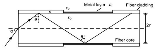
Figure 1. Light transmission mode in an optical fiber.
