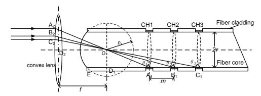
Figure 6. Proposed design of a novel multi-channel fiber-optic SPR sensor.
