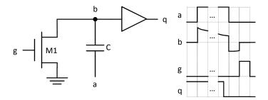
Since the value at which the node is charged is variable due to the process fluctuations, clock skew and jitter, an extra buffer was introduced at the output of the sensor with a threshold above that of the first buffer, as shown in Figure 2. In this way, there is an extended control over the measurement interval, since both  $V_1$  and  $V_2$  are fixed by the buffers.
