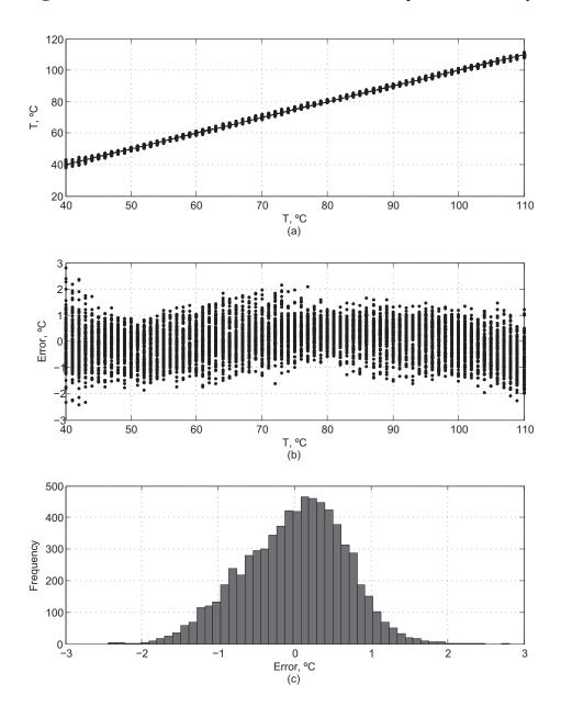
In order to estimate the effects of fabrication uncertainties on our sensor, we have performed 100 Monte Carlo simulations considering process variations and mismatches. The vendor provides a description of the probability distribution for each parameter of the transistor model. The electronic design automation (EDA) tool produces a cloud of values for each parameter accordingly to their probability distributions, so that a set of 100 test circuits—representing different technology corners—are
