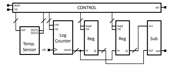
**Figure 5.** Constituent blocks of the 65 nm thermal sensor.
