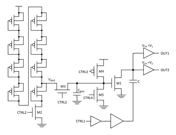
**Figure 2.** Complete sensing part schematic.
