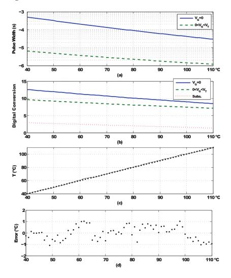
Figure 7a-d shows the results of the sensor characterization performing post-place-and-route simulations and taking one sample for each integer in the range. The variation of the pulse widths
