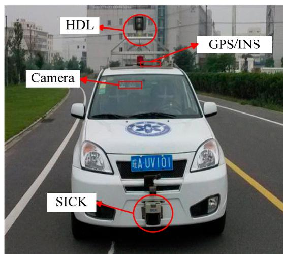
The system architecture of “Intelligent Pioneer” is a distributed architecture [31]. It can be divided into five subsystems: environment perception system, decision making system, sensor system, control system, and the actuators. These subsystems are connected through Ethernet for inter-subsystem communication.
