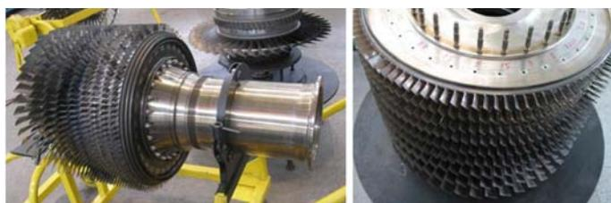
**Figure 5.** Photograph of the dismountable disk-drum aero-engine rotor.
