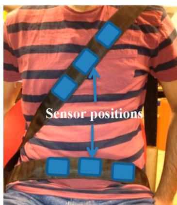
**Figure 1.** Subject wearing the prototype safety belt.
