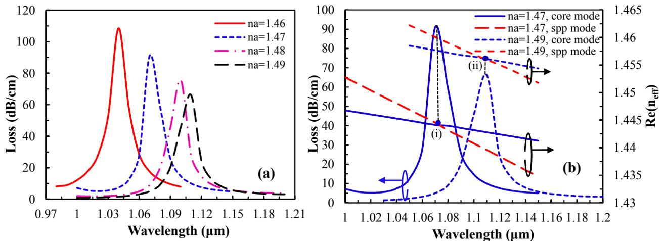
**Figure 3.** (a) Loss spectrum of the fundamental mode by increasing analyte RI,  $n_a$ , from 1.46 to 1.49; (b) dispersion relation of the core-guided mode for  $n_a = 1.47$  (solid lines) and  $n_a = 1.49$  (dashed lines). Red and blue lines indicate SPP mode and the fundamental core-guided mode respectively. Point (I) and (II) are the phase matching points for analyte  $n_a = 1.47$  and 1.49.
