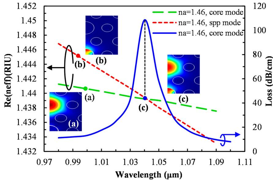
**Figure 2.** Dispersion relation of the core-guided mode (green), plasmonic mode (red) and the loss spectrum (blue); inset (a,c) show the electric field of the core-guided mode and inset (b) shows the electric field of the plasmonic mode.
