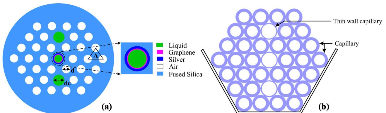
**Figure 1.** (a) Cross-section of the proposed sensor; (b) Cross-section of the stacked preform.
