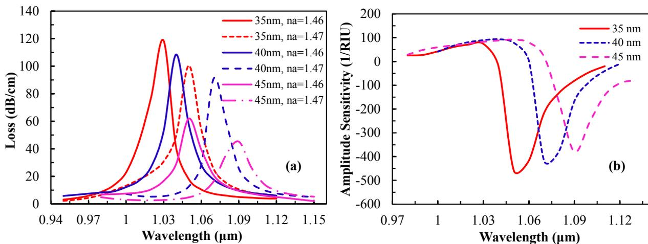
**Figure 5.** (a) Loss spectrum and (b) amplitude sensitivity vs. wavelength by varying silver thickness, setting analyte RI at  $n_a = 1.46$ .
