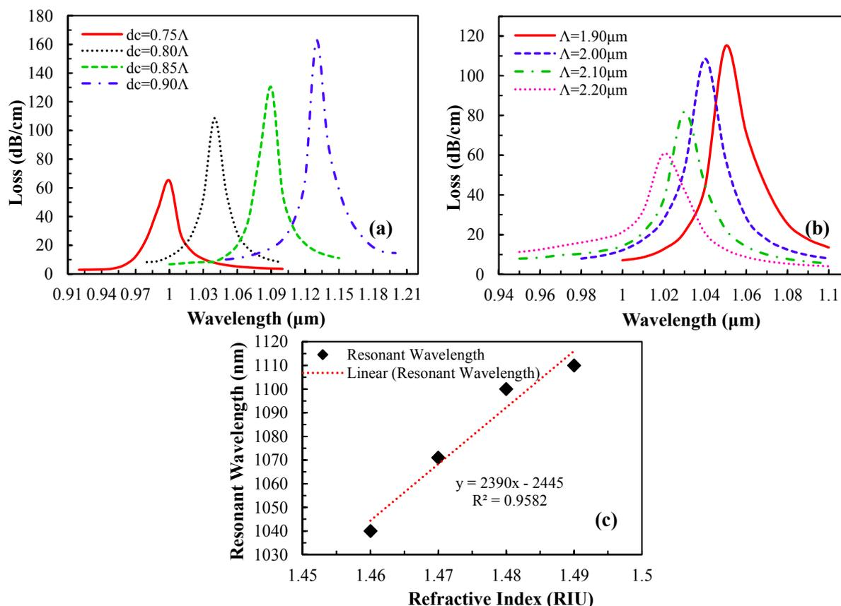
**Figure 7.** Loss spectrum vs. wavelength with the variation of (a) metallic core diameter  $d_c$ , (b) pitch size  $\Lambda$  (analyte RI,  $n_a = 1.46$ ) and (c) linear fitting of the fundamental mode resonant wavelength vs. analyte RI.
