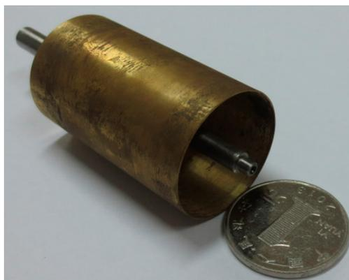
**Figure 4.** The entity of the cup rotor.
