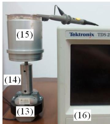
**Figure 18.** Connection diagram of a single-phase asynchronous motor angular acceleration testing.
