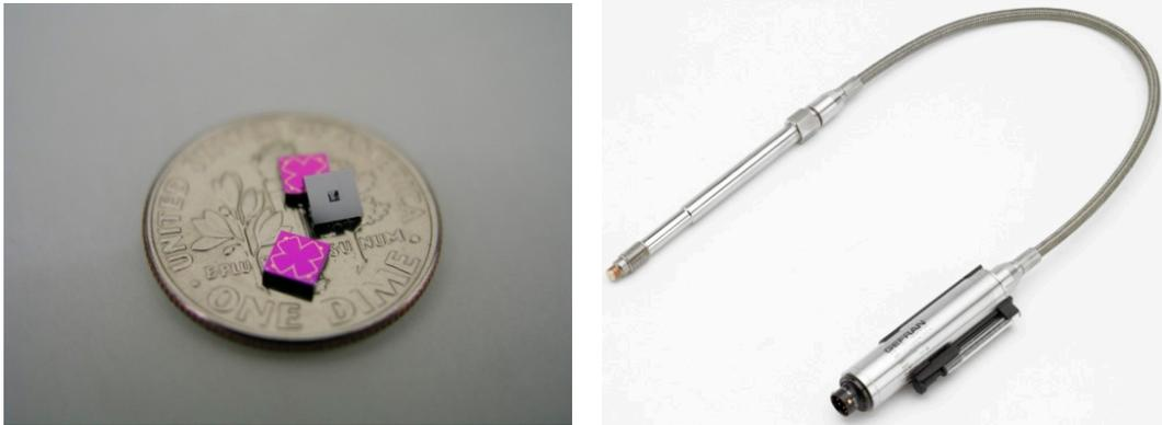
**Figure 5.** Fabricated SOI chips for floating concept. The chip size is  $3.6 \times 3.6 \text{ mm}^2$ , compared with one dime coin (**left**). Packaged sensor system for use in plastic injection application (**right**) [8].
