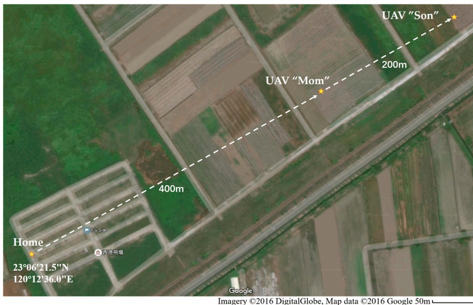
**Figure 21.** Final positions of nodes in the Google map in the extended distance test in Taiwan.
