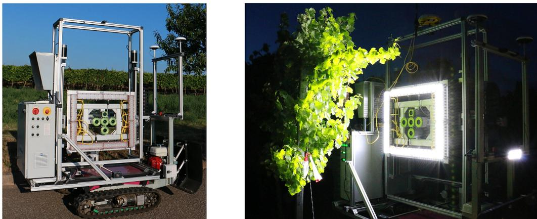
**Figure 4.** The PHENObot. RTK-GPS is attached at the top. A five camera system is attached on a camera movement frame to adjust the camera-canopy distance and camera height. The RGB camera in the middle of the camera system was used for our purposes. Around the camera system, the lighting unit is situated in a rectangular frame.
