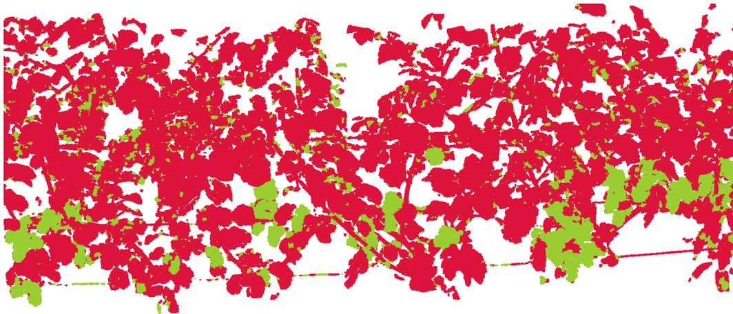
**Figure 10.** Classified point cloud after label smoothing. Former heterogeneous regions are now homogeneous. Small regions of misclassified points are corrected. Branches lying in between grape bunches are classified correctly.
