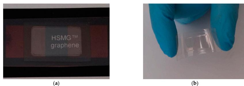
**Figure 4.** Examples of fully transparent temperature sensors: (a) transparency of cryogenic sensor—photo of the sensor on a black background with a white label; (b) stretchability of the sensor.
