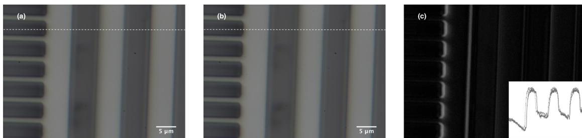
**Figure 7.** Images from the optical microscope of the grating beams (a) before the application of the voltage; (b) with the application of voltage; (c) difference between the two images (the inset shows a line plot along the dashed line in (a,b)).
