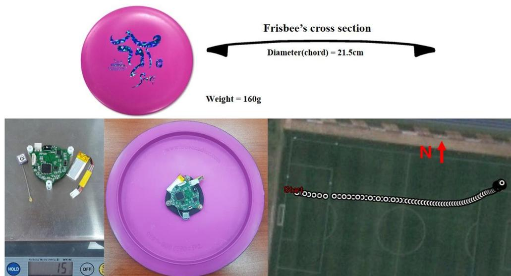
**Figure 10.** Disc and onboard sensor module for the field experiment.
