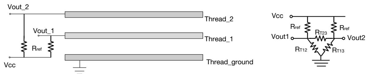
Figure 4. Sensor output circuit.
