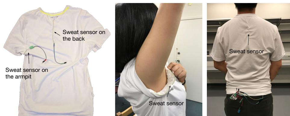
**Figure 15.** On-body experiment settings and sensor calibration. Two sweat sensors were sewn into a shirt at similar locations to conduct the sensor calibration before beginning the human experiments.
