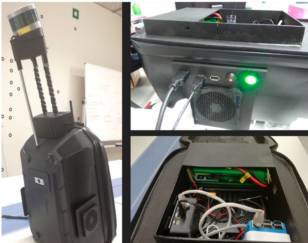
**Figure 1.** (Left) General view of the wearable prototype. (Right) Detail of the interior of the wearable prototype.
