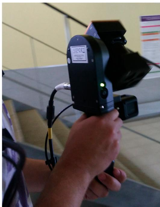
**Figure 6.** View of the Zeb-Revo during acquisition.
