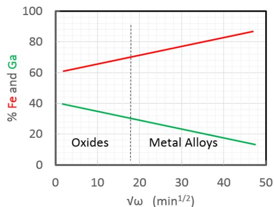
**Figure 4.** Due to differences in mass transport rates, the composition of Gafenol films can be tailored simply using the rotation rate ( $\omega$ ) of a rotation disk electrode [14].
