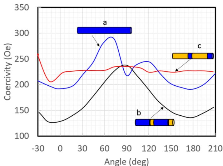
**Figure 11.** The coercivity from magnetic hysteresis loops for (a) pure Galfenol nanowires and segmented Galfenol/Cu nanowires with (b) 50 nm of Cu in Galfenol nanowires or (c) 50 nm Galfenol in Cu nanowires (diameter = 100 nm; long segments 400 and 500 nm, respectively).
