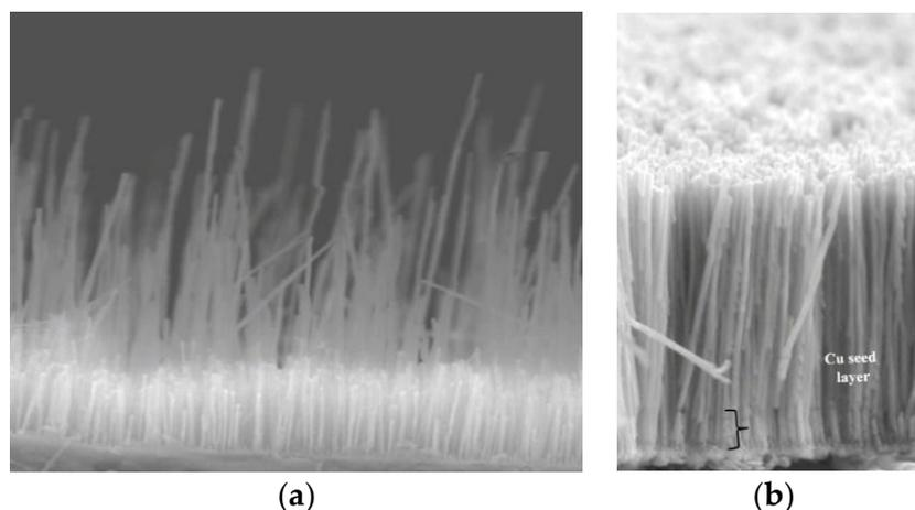
**Figure 9.** (a) A second problem unique to Galfenol was extremely inhomogeneous lengths, where many short nanowires ( $\sim 4 \mu\text{m}$ ) were seen at the growth electrode while others grew extremely fast, even to the top of the template. (b) Uniform lengths ( $8 \mu\text{m} \pm 3\%$ ) were achieved using a rotating disk electrode, a Cu seed layer, and pulsed deposition [20].
