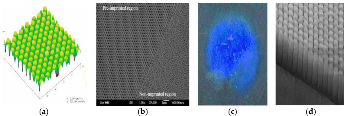
**Figure 10.** (a)  $\text{Si}_3\text{N}_4$  nanostamp to imprint Al films and foils so that (b) nanopores aligned in the subsequent oxide formed by anodization of the Al. (c) Line stamps of Ni could be made large enough to use for large area (1 cm in diameter) alignment, shown diffracting blue light. (d) Magnification of nanopores (1  $\mu\text{m}$  long) produced by line stamps [23,26].
