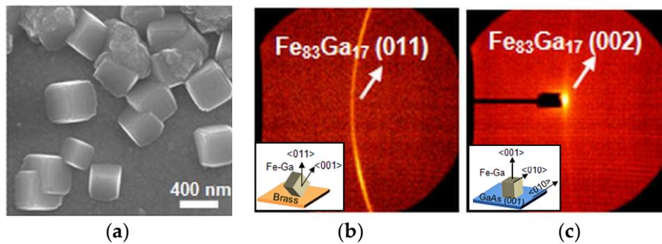
**Figure 5.** Galfenol grown with slow deposition rates onto (a) brass substrates, resulting in (b) primarily cube on edge texturing. (c) Although some grains were observed with low-energy (110) orientations, a majority of the grains were epitaxially oriented on GaAs. Reproduced from [13], with the permission of AIP Publishing.
