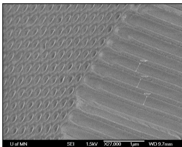
**Figure 7.** Anodic aluminum oxide template [19].
