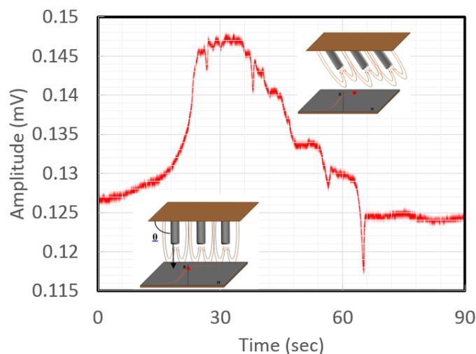
**Figure 12.** Signal from magnetoresistive sensors at the bottom of a microfluidic channel showing a direct proportionality to flow due to a rapid increase in pressure then a slow release with three sudden drops in pressure and a final backwash from complete pressure release [36].
