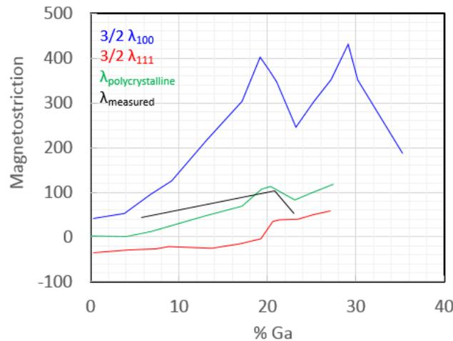
**Figure 6.** Measured values for the magnetostriction of Galfenol crystallographic orientations and the calculated value of polycrystalline Galfenol, which compares well to measured values [17].
