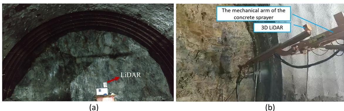
**Figure 4.** The LiDAR in the real tunnel. (a) Data collection site; (b) practical application.
