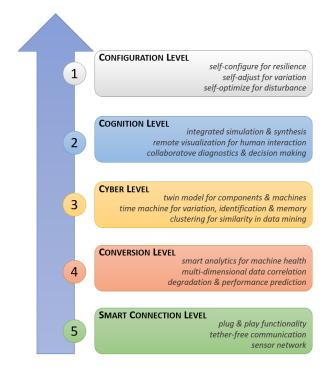
**Figure 2.** Five-layer architecture of CPS implemented in industrial settings. Lower levels collect data, which is analyzed and condensed at each upper level. With this configuration, information fed to each higher level is more valuable than information coming into the level below.
