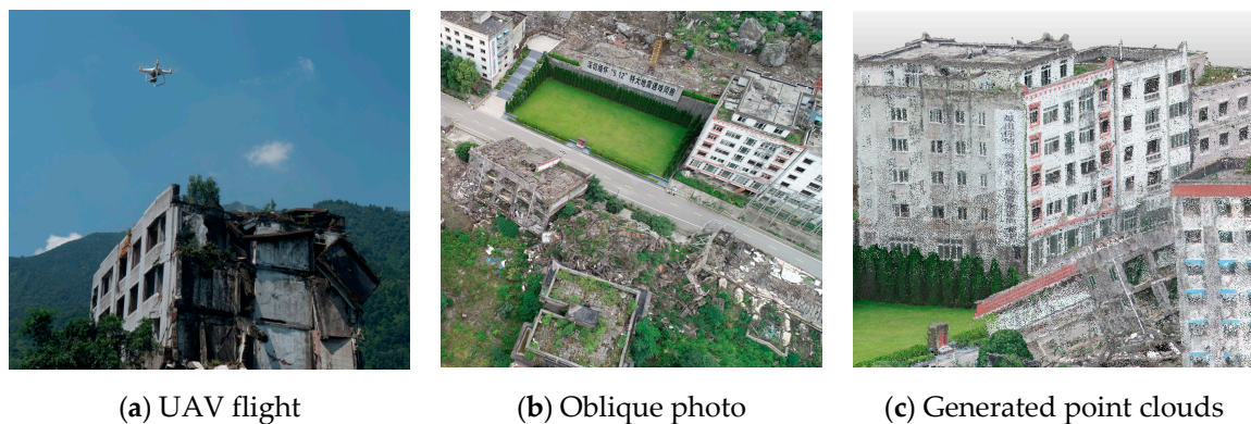
Figure 3. UAV data acquisition and some data products.
