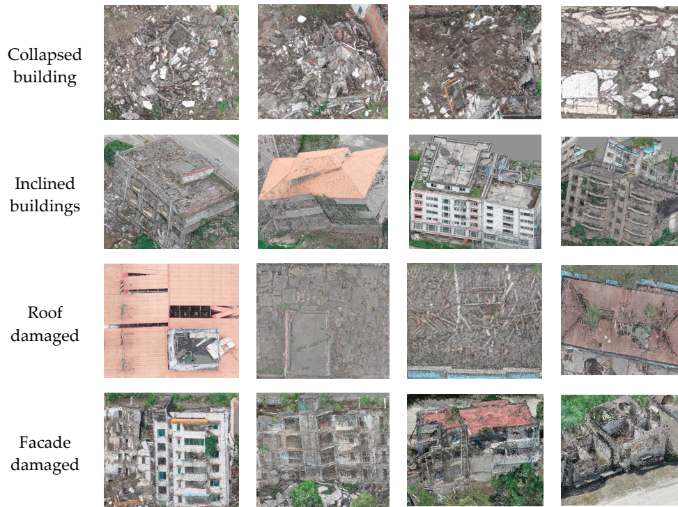
Figure 8. Representative damage samples based on different damage features.
