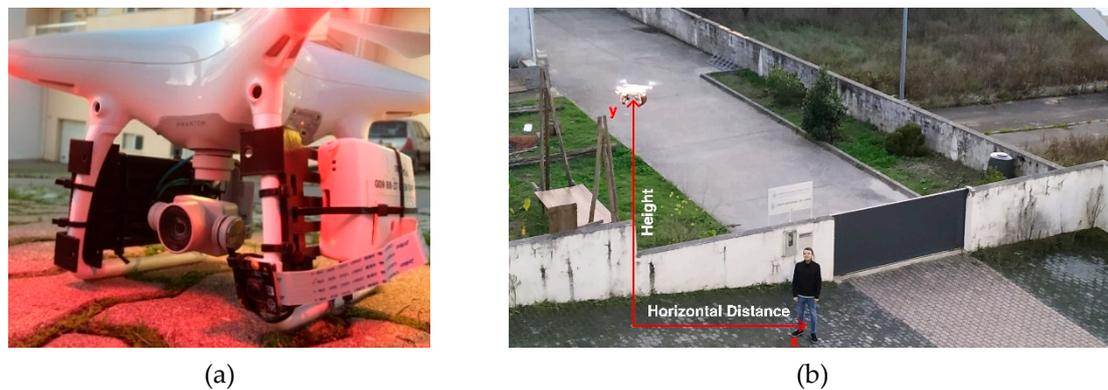
**Figure 15.** (a) Picture of the DJI Phantom 4 with the Raspberry Pi 3 microcomputer, camera and the power bank; (b) representation of the third test scenario, with the drone carrying Raspberry Pi.
