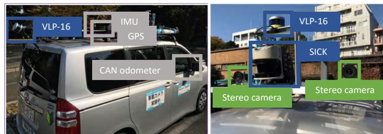
**Figure 5.** Experimental vehicle. Two sixteen-layer laser scanners (VLP-16) and one single-layer laser scanner were mounted for the point cloud map generation. One of the VLP-16s was used for self-localization in our experiments. Furthermore, the single-layer scanner, LMS511, was used to collect the reflection intensities of the LiDAR scans.
