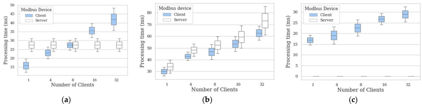
**Figure 5.** Processing time of (a) registration phase; (b) channel securing phase; (c) verification phase.
