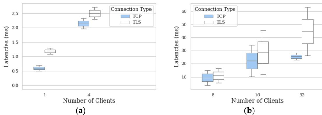
**Figure 6.** Latencies' measurements in the fourth phase for the following architectures: (a) 1:1 and 4:1; (b) 8:1, 16:1 and 32:1.
