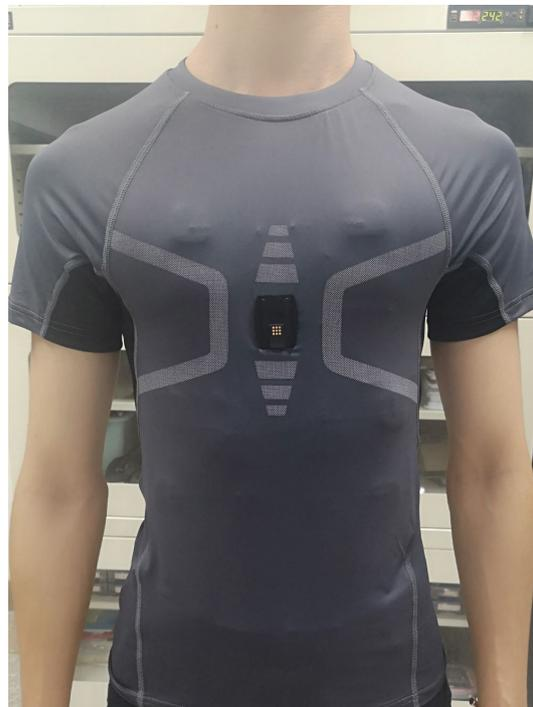
**Figure 1.** A wearable ECG device that collects the ECG signals through three embedded fabric electrodes in the vest.
