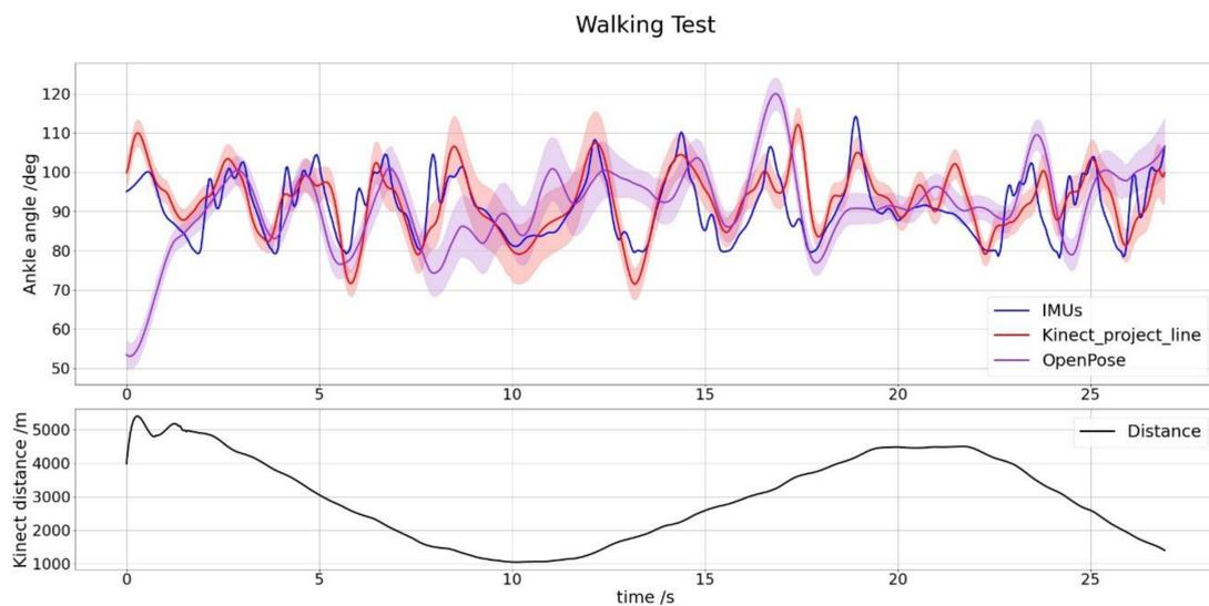
**Figure 17.** Graph showing the comparison between the ankle angle measured by the Kinect v2 with our projection lines method (red), the ankle angle measured by OpenPose (violet) and the angle measured by the IMUs using Euler's angles (blue), for the walking test. Red and violet shaded area is the Kinect angle error following Equation (20). The body distance average is shown below to complete the information.
