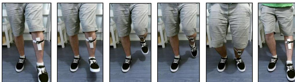
**Figure 1.** Example of frames from a recording of the Kinect v2 measuring simultaneously with the inertial measurement units (IMUs), one on the foot and one on the leg below the knee, for the calculation of the ankle angle. Distance of 0.5 m. Only shows the region of interest for each frame.
